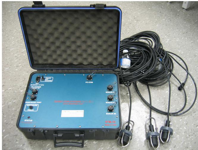
Figure 1.3: Pilot acoustic positioning system.
