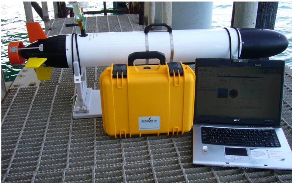
Figure 7.1: Picture of the Iver2 AUV.
