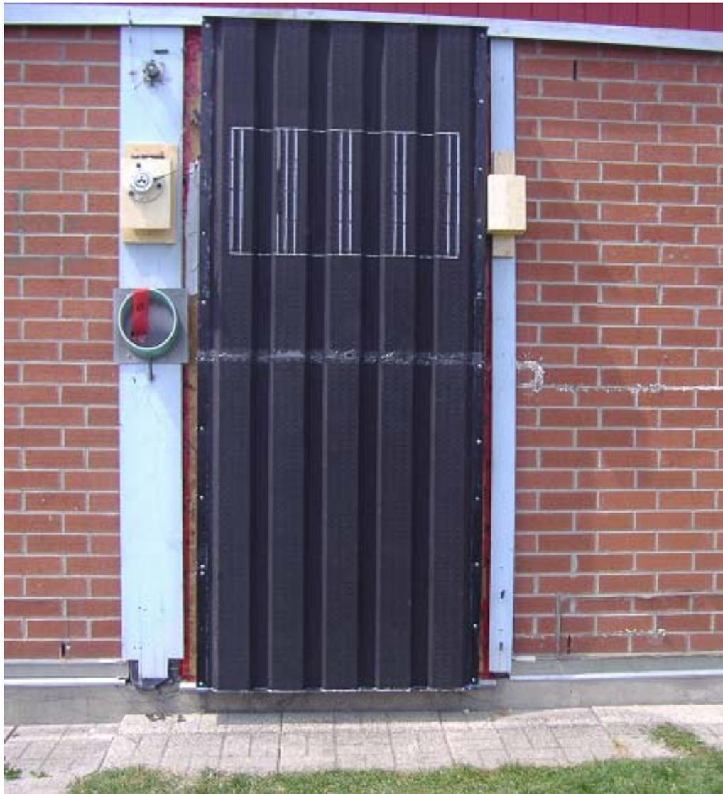
**Figure 4.7:** PV/Thermal transpired solar collector prototype installed on the BEG Hut east facing wall
