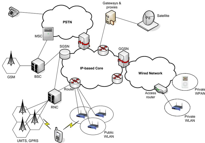
Figure 1.1: An architecture of next-generation all IP-based wireless networks.
