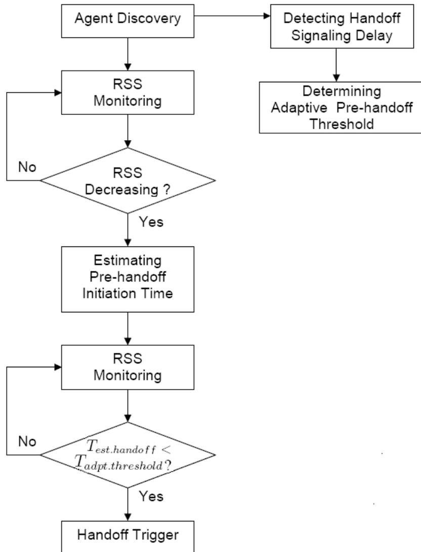
Figure 3.7: Flow chart diagram of the the proposed handoff scheme
