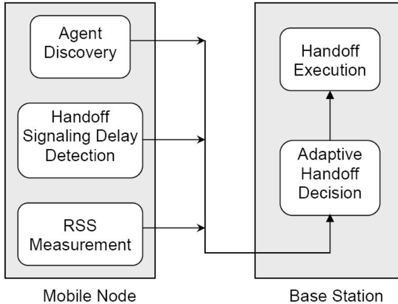
Figure 3.5: Architecture of the proposed handoff scheme
