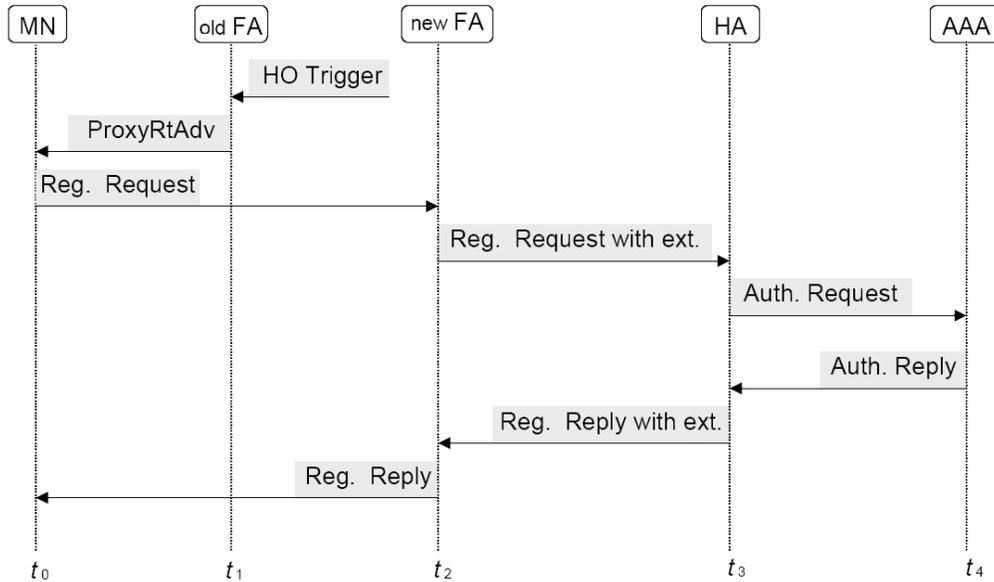
Figure 3.8: Timing diagram for the proposed handoff scheme
