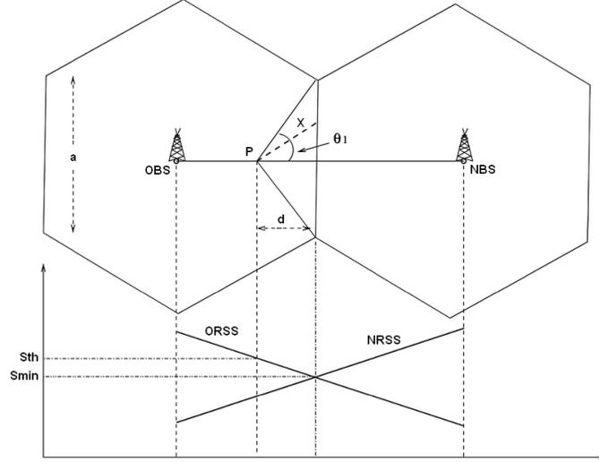
Figure 3.1: A typical handoff process
