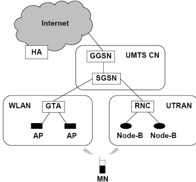
Figure 2.3: Tight coupling architecture.
