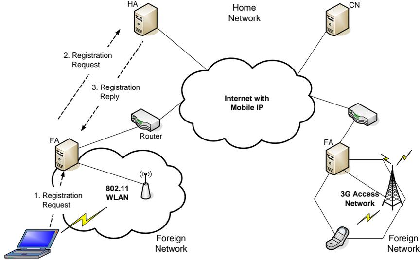
Figure 2.4: Mobile IP network architecture.
