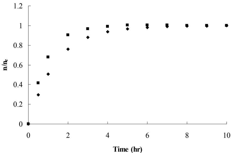
**Figure 6-14** Extraction profiles in the sample matrix with the same free concentration of analyte. (■) with the presence of binding matrix; (◆) without the presence of binding matrix.
