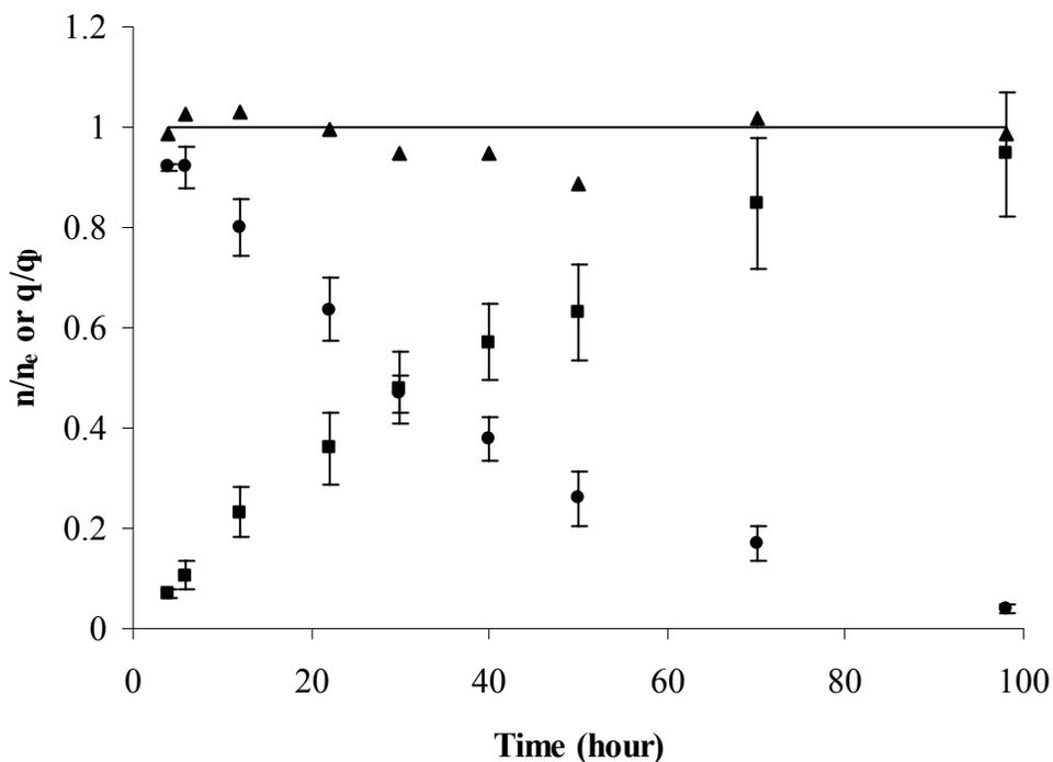
**Figure 3-5** Absorption and desorption profiles in PDMS rod. Simultaneous absorption of pyrene (■) onto the PDMS rod from the flow through system and desorption of deuterated pyrene (●) from the PDMS rod into the flow-through system. (▲) represents of the sum of  $Q/q_0$  and  $n/n_e$
