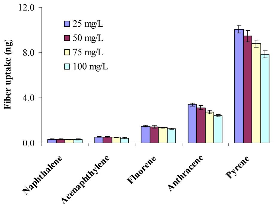
Figure 4-7 Comparison of fiber uptake at different concentrations of fulvic acid (n=3).
