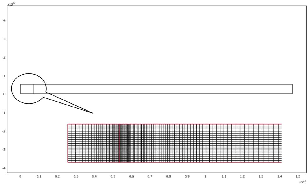
**Figure 6-2** Schematic diagram of model domain and mesh generated for static sample.
