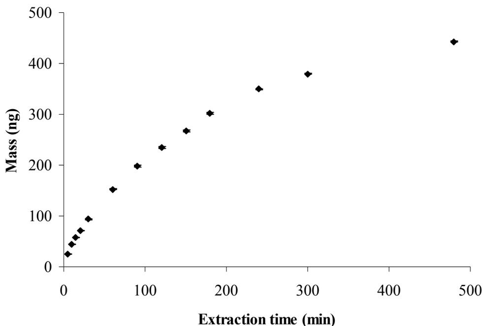
**Figure 2-2** Extraction profile of solid pyrene containing in a vial (n=5).
