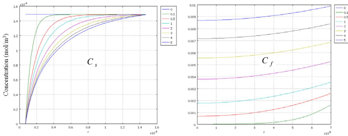
**Figure 6-10** Concentration distribution profile in sample ( $C_s$ ) and in fiber coating ( $C_f$ ) at different extraction times from 0 to 5 s.
