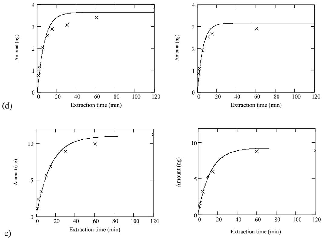
Appendix 3 Extraction profiles of PAH in aqueous solution with (right column) and without (left column) NOM. (a) naphthalene; (b) acenaphthylene; (c) fluorene; (d) anthracene; and (e) pyrene.
