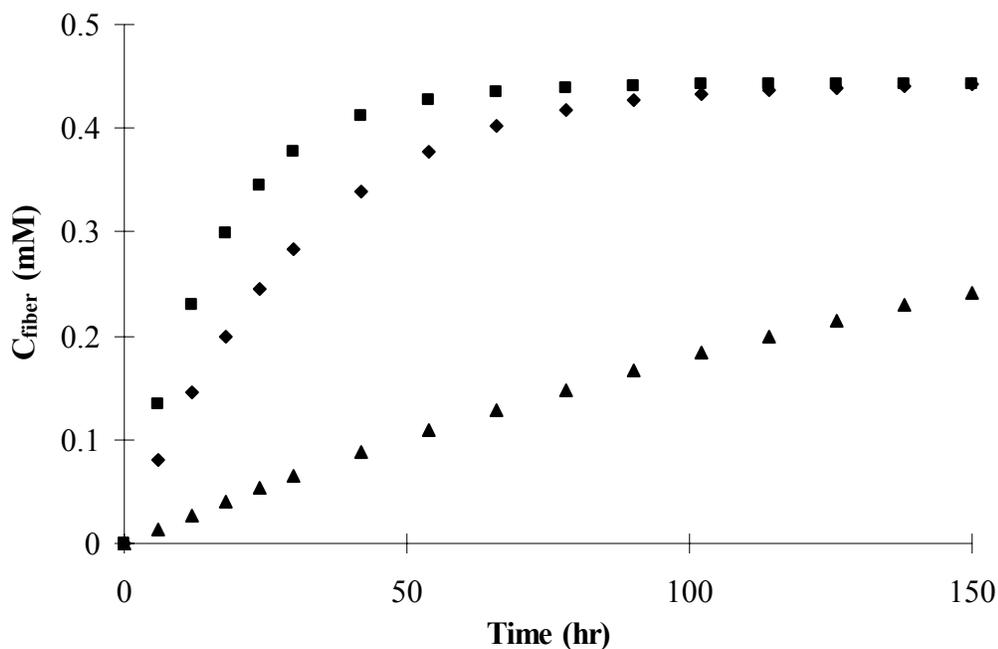
**Figure 6-16** Extraction profiles at different flow velocities. (■)  $1.7 \times 10^{-4}$  m/s, (◆)  $8.5 \times 10^{-5}$  m/s and (▲)  $8.5 \times 10^{-6}$  m/s.
