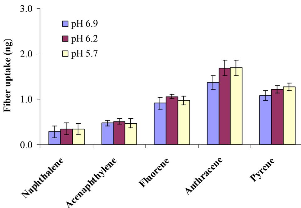
**Figure 4-4** Fiber uptakes at different pHs of sample-matrix with humic acid (Sigma-Aldrich) (n=3).
