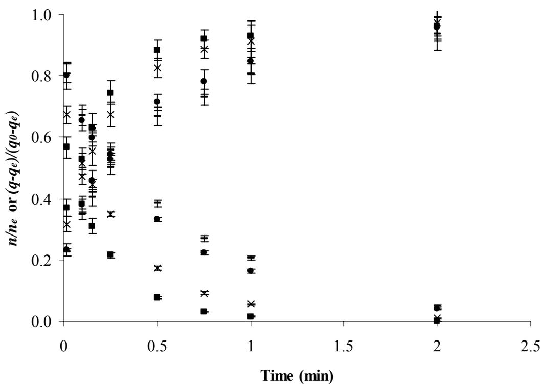
**Figure 2-3** Absorption and desorption profiles of BTEX at 25 °C. Benzene(■); toluene (×); ethylbenzene (●) and *o*-xylene (◡).
