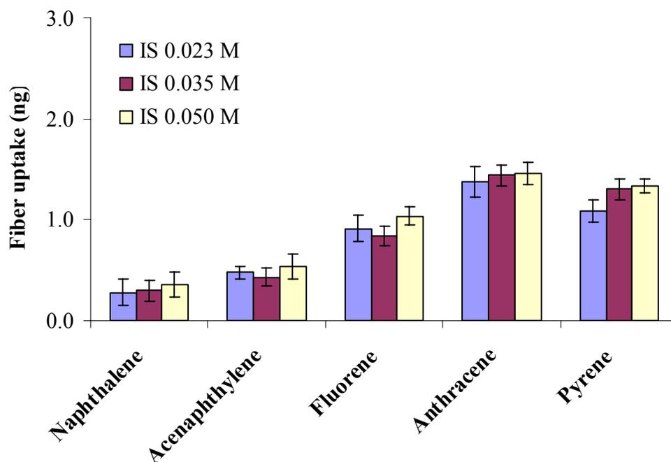
**Figure 4-5** Fiber uptakes at different ionic strengths of sample matrix with humic acid (Sigma – Aldrich) (n=3).
