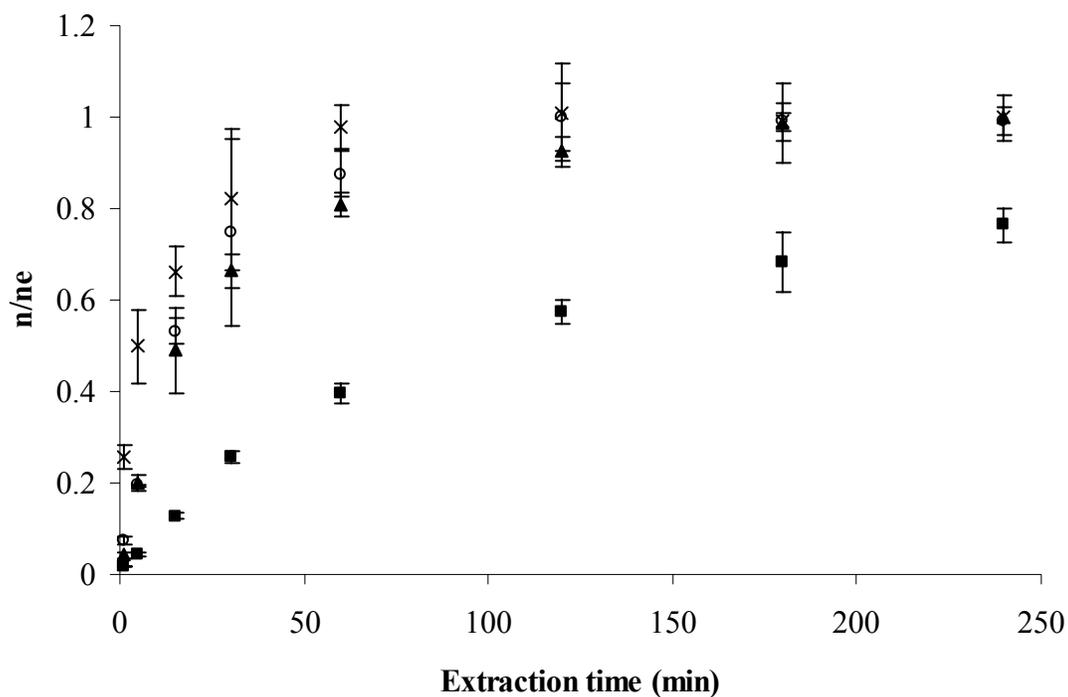
**Figure 5-6** Extraction profiles at the static and agitation condition. Fluorene: static condition (○), 500 rpm (×); Pyrene: static condition (■), 500 rpm (▲).
