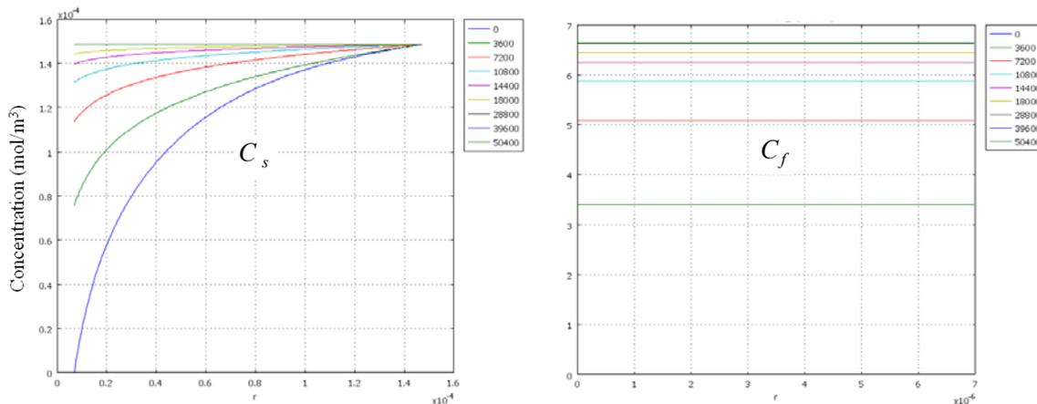
**Figure 6-11** Concentration distribution profile in sample ( $C_s$ ) and in fiber coating ( $C_f$ ) at different extraction times from 0 to 15 hrs.
