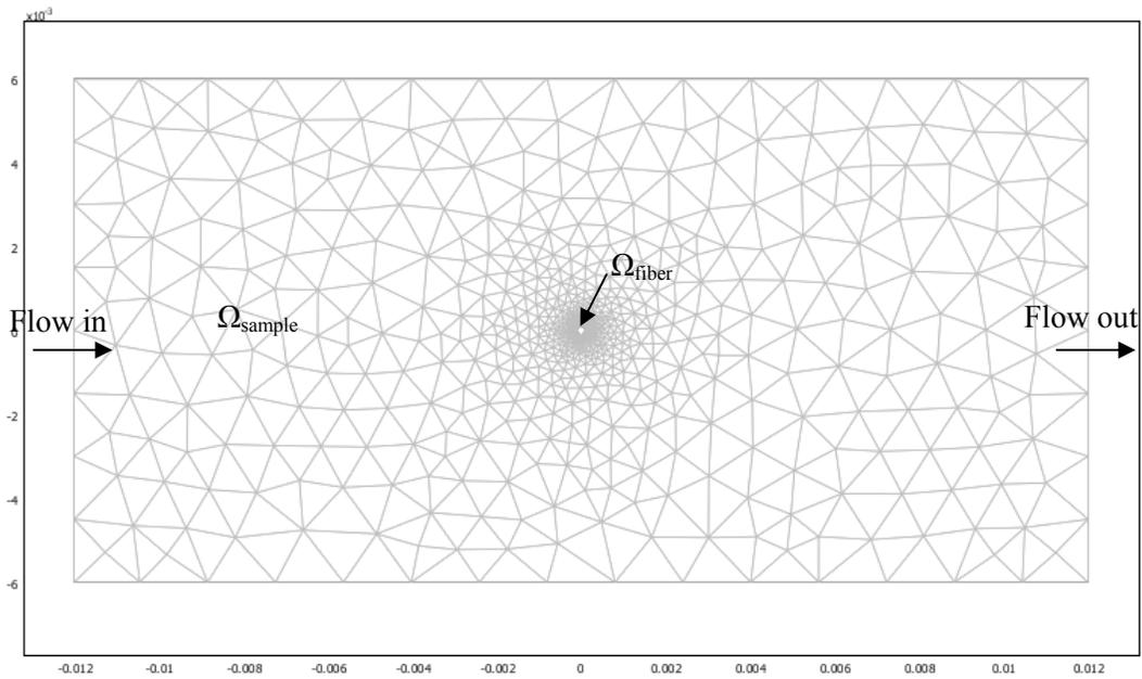
**Figure 6-3** Schematic diagram of model domain and mesh generated for flow-through system.
