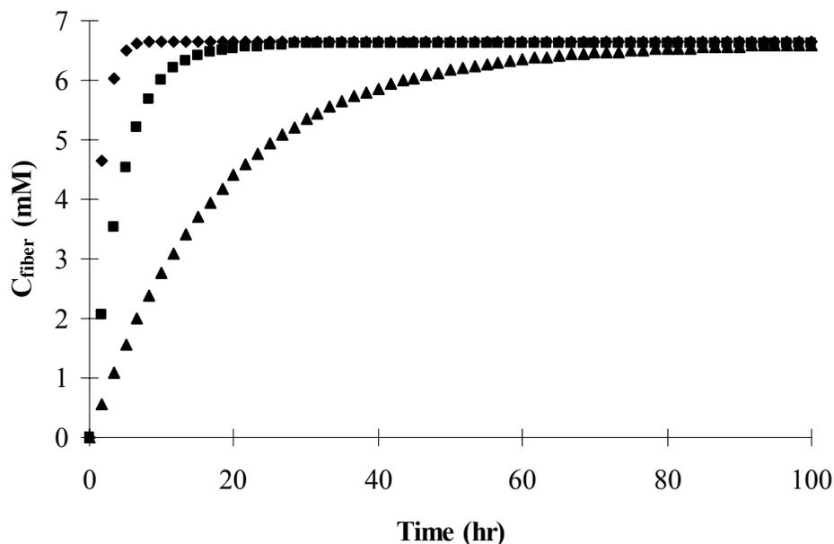
**Figure 6-13** Extraction profiles with different thickness of fiber coatings. (◆) 7  $\mu\text{m}$ , (■) 14  $\mu\text{m}$  and (▲) 35  $\mu\text{m}$ .
