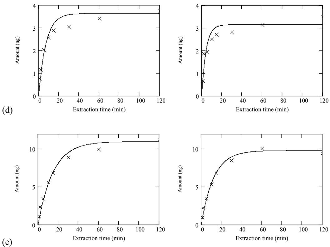
Appendix 2 Extraction profiles of PAH in aqueous solution with (right column) and without (left column) fulvic acid. (a) naphthalene; (b) acenaphthylene; (c) fluorene; (d) anthracene; and (e) pyrene.
