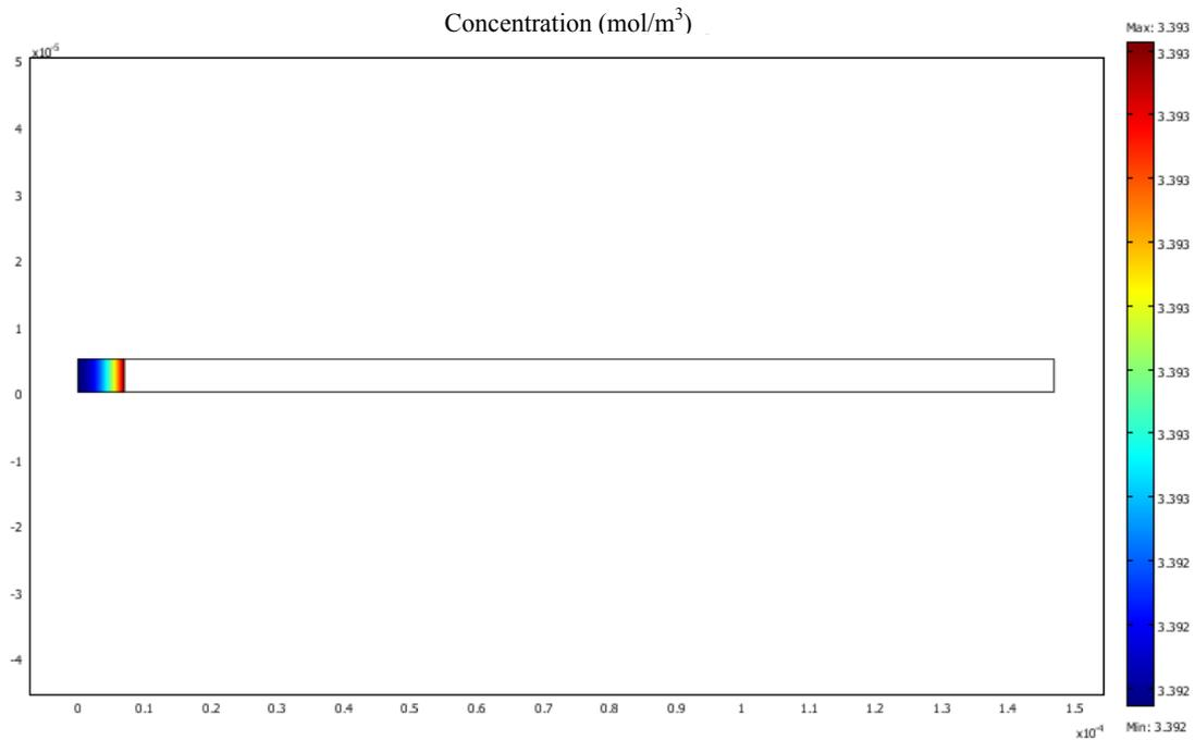
**Figure 6-8** Surface concentration profile on the fiber coating at  $t = 60$  min.
