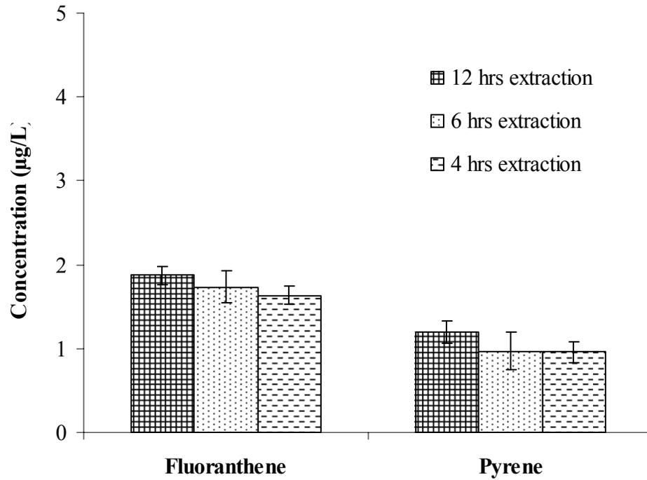
**Figure 3-6** Comparison of the estimated concentrations of fluoranthene and pyrene in the flow-through system with different sampling times.
