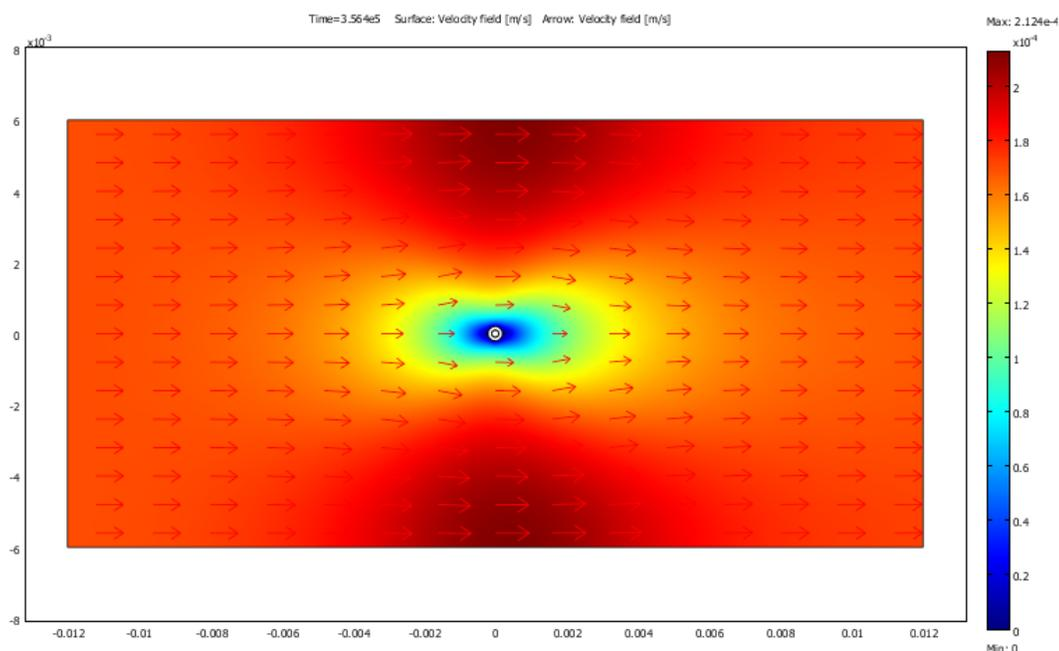
**Figure 6-15** The flow pattern around the fiber coating. The colour bar represents the modulus of the velocity vector, while the arrows symbolize the flow velocity vector.
