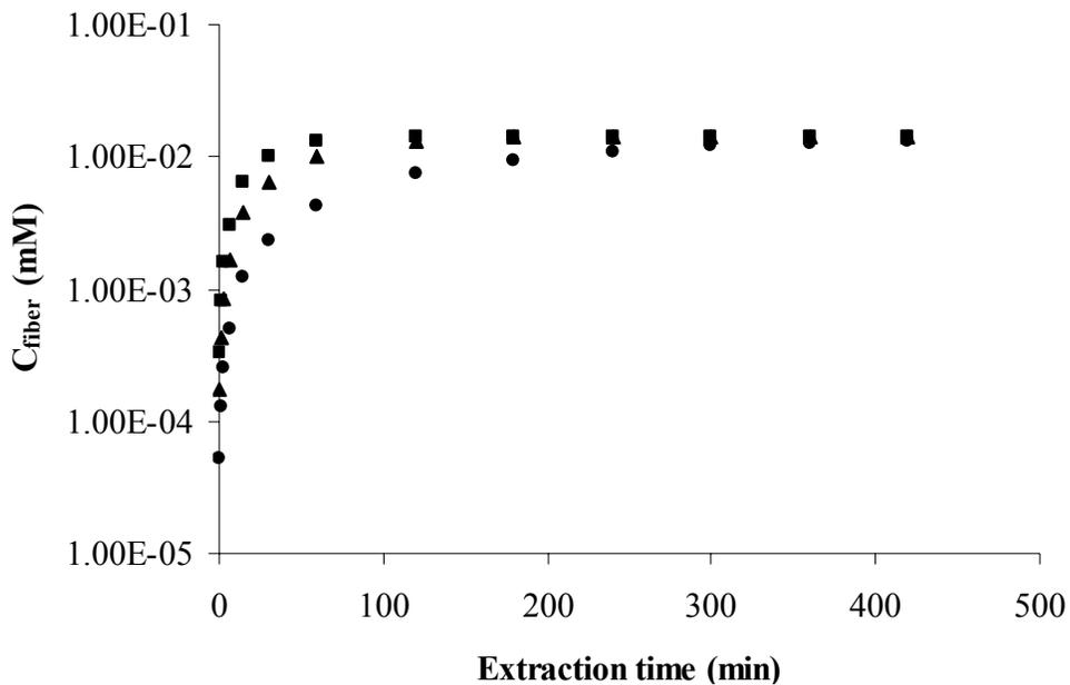
Figure 5-3 Extraction profiles at different agitation condition: 1200 rpm (■), 600 rpm (▲) and 100 rpm (●).
