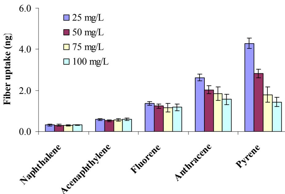
**Figure 4-6** Comparison of fiber uptake at different concentrations of humic acid (n=3).
