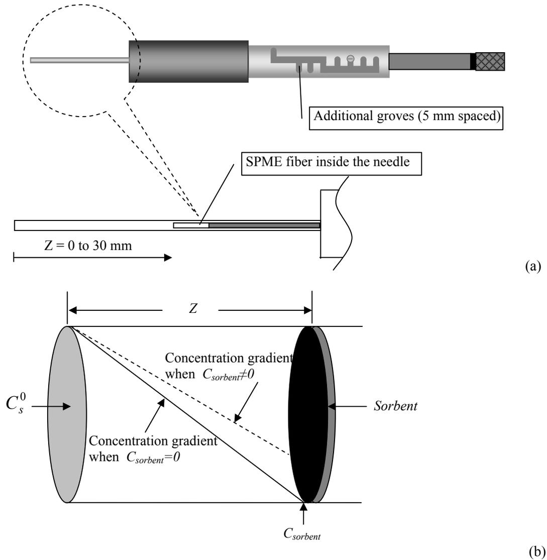
**Figure 1-5** Use of SPME for in-needle time-weighted average sampling: (a) adaptation of commercial SPME manual extraction holder; (b) schematic diagram of fiber retracted SPME device and concentration gradient.
