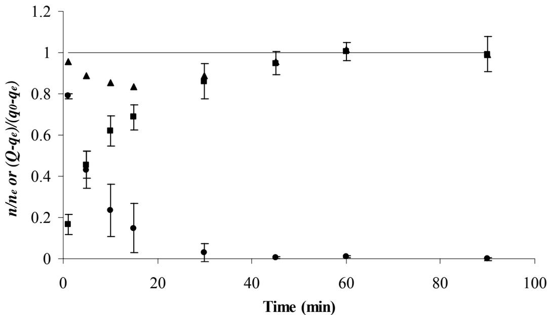
**Figure 5-7** Absorption and desorption profiles in SPME fiber in the complex sample matrix with humic acid. Simultaneous absorption of pyrene (■) onto the PDMS fiber and desorption of deuterated pyrene (●) from the PDMS fiber. (▲) represents of the sum of  $\frac{Q - q_e}{q_0 - q_e}$  and  $\frac{n}{n_e}$ .
