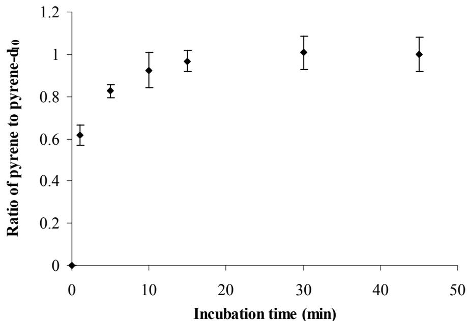
**Figure 4-1** Sorption kinetics of pyrene onto humic acid (Sigma-Aldrich) (n=2).
