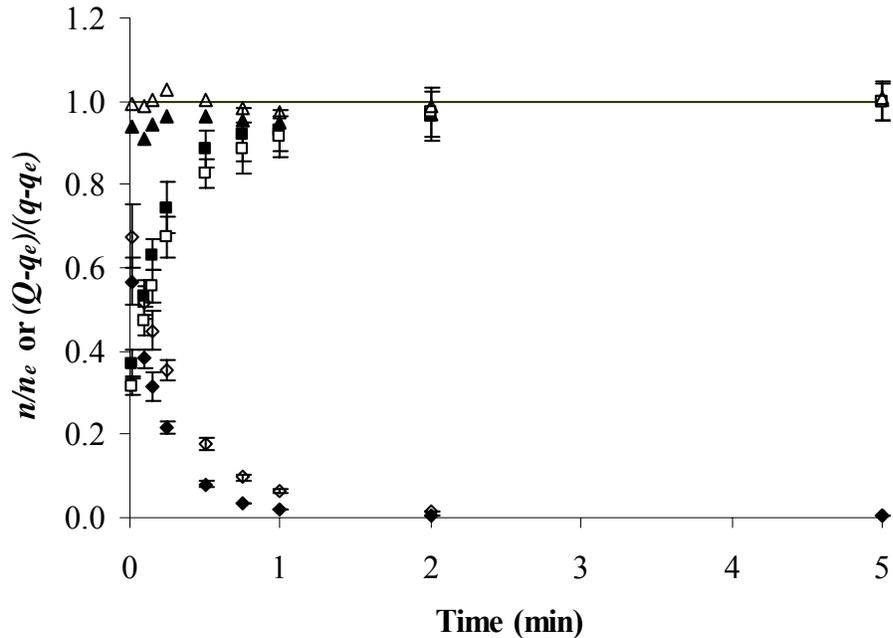
**Figure 2-4** Absorption and desorption profiles in SPME. Simultaneous absorption of benzene (■) and toluene (□) and desorption of benzene-*d*<sub>6</sub> (◆) and toluene-*d*<sub>8</sub> (◇); (▲) and (△), the sum of  $n/n_e$  and  $(Q - q_e)/(q_0 - q_e)$  for benzene and toluene.
