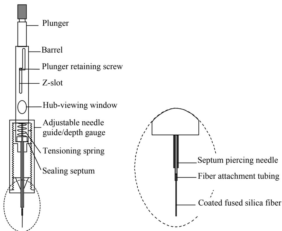
**Figure 1-2** Design of the first commercial SPME device made by Supelco.
