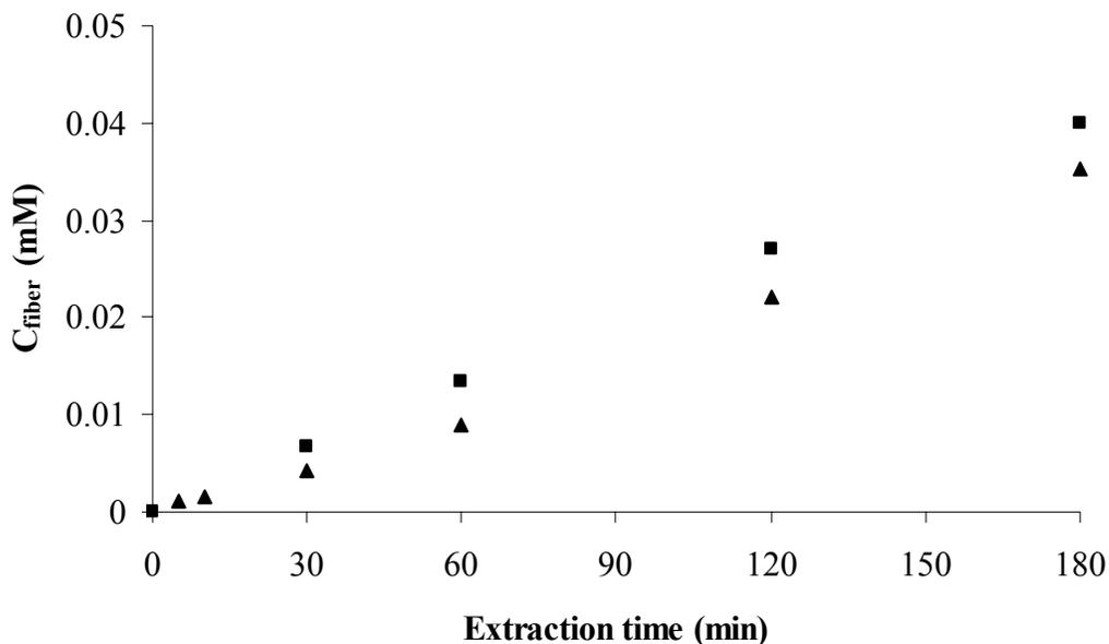
**Figure 6-18** Comparison of extraction profiles from simulation results and experimental data. (■) simulation results and (▲) experimental data (Flow velocity =  $8.5 \times 10^{-5}$  m/s).
