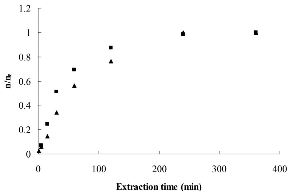
**Figure 6-17** Comparison of extraction profiles from simulation results and experimental data. (■) simulation results and (▲) experimental data (Static sample).
