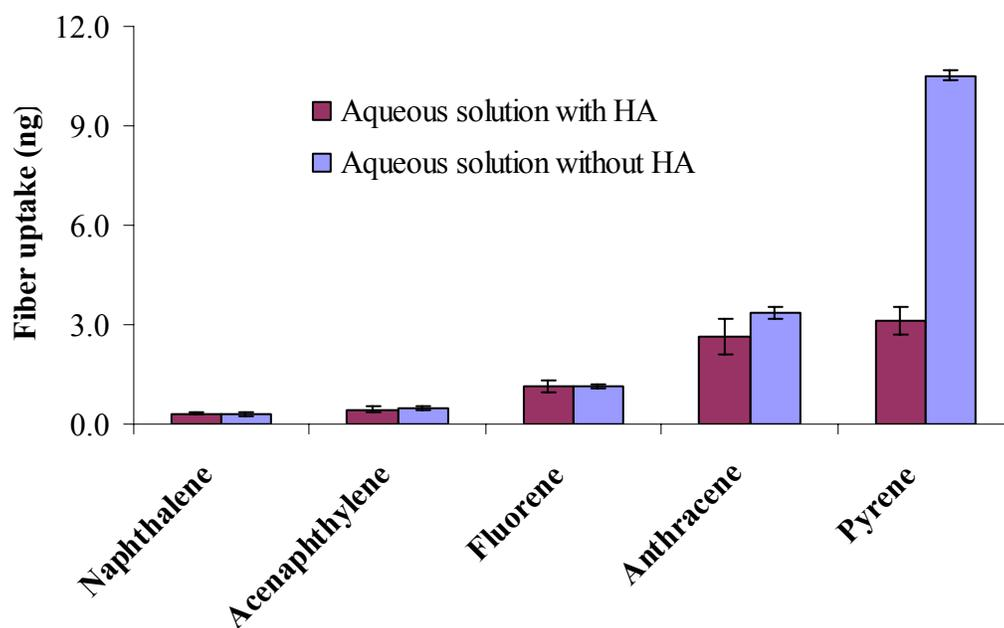
**Figure 4-3** Fiber uptakes of PAHs by SPME in aqueous samples with or without humic acid (n=3).
