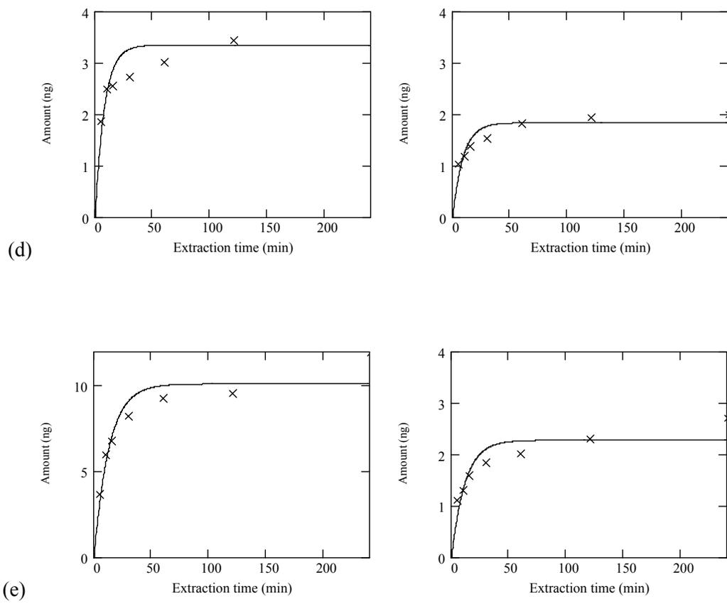
Appendix 1 Extraction profiles of PAH in aqueous solution with (right column) and without (left column) humic acid. (a) naphthalene; (b) acenaphthylene; (c) fluorene; (d) anthracene; and (e) pyrene.
