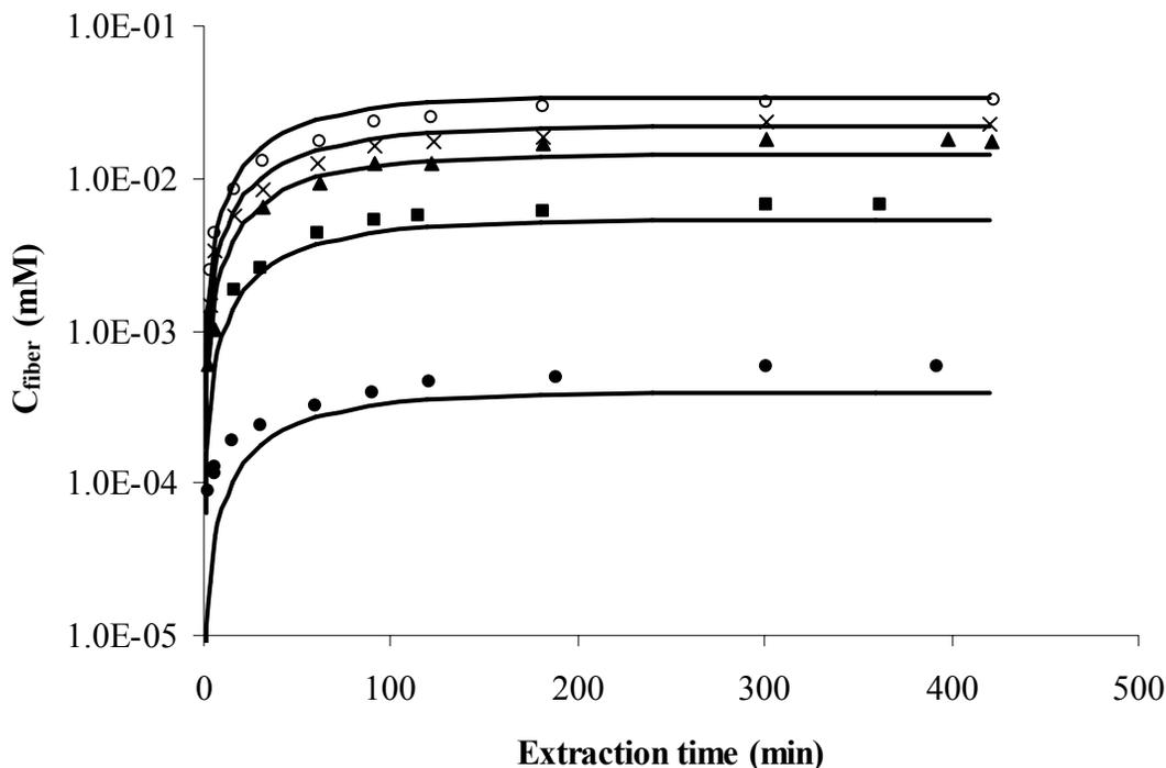
**Figure 5-1** Extraction profiles of [<sup>3</sup>H]estradiol at different BSA concentrations: 0 M (○),  $6.5 \times 10^{-6}$  M (×),  $1.6 \times 10^{-5}$  M (▲),  $6.4 \times 10^{-5}$  M (■) and  $1.0 \times 10^{-3}$  M (●). The curves are drawn based on the calculation results from the kinetic model.
