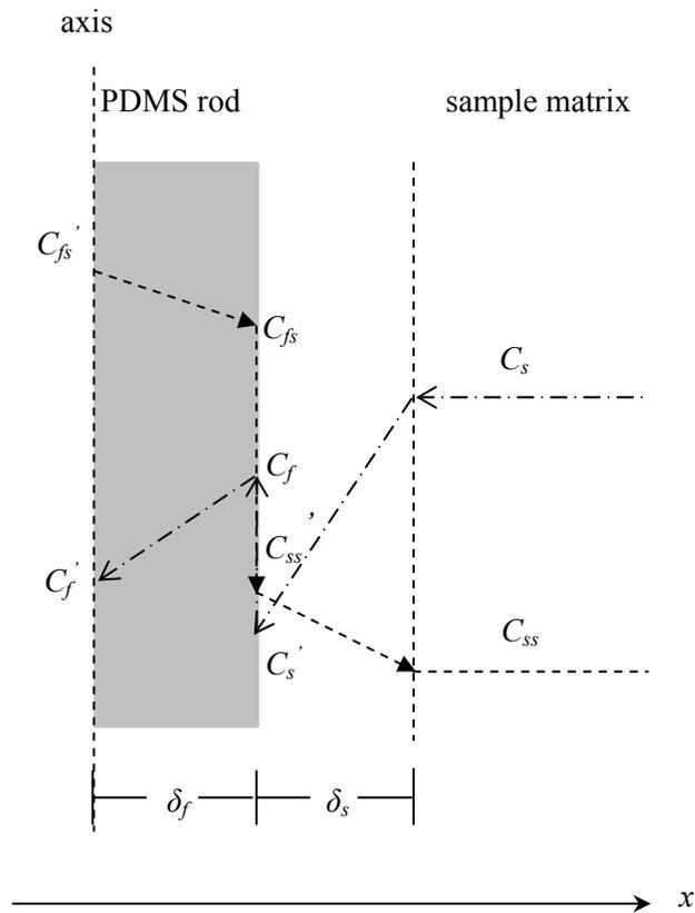
**Figure 3-2** Schematic of the calibration of the extraction of target analyte by the desorption of a standard from a PDMS rod to an aqueous media in field sampling.
