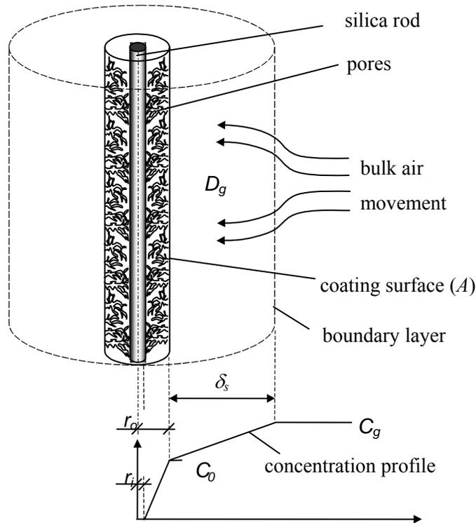
**Figure 1-4** Schematic diagram of the diffusion-based calibration model for cylindrical geometry.
