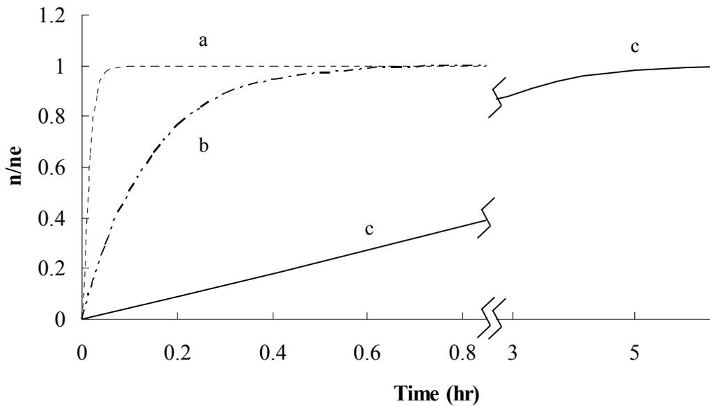
**Figure 6-12** Extraction profile with different distribution coefficients. (a)  $\log K_{fs} = 2.65$ , (b)  $\log K_{fs} = 3.65$  and (c)  $\log K_{fs} = 4.65$ .
