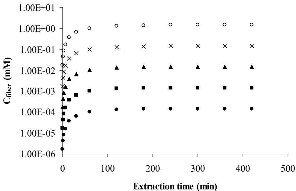
**Figure 5-2** Extraction profiles at different total analyte concentrations:  $7.11 \times 10^{-7} \text{ M}$  (○),  $7.11 \times 10^{-8} \text{ M}$  (×),  $7.11 \times 10^{-9} \text{ M}$  (▲),  $7.11 \times 10^{-10} \text{ M}$  (■) and  $7.11 \times 10^{-11} \text{ M}$  (●).
