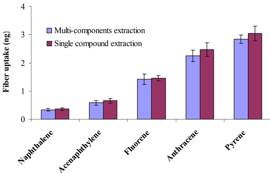
**Figure 4-2** SPME uptakes from solutions containing one component and multi-components in the presence of humic acid (Sigma – Aldrich) (n=3)
