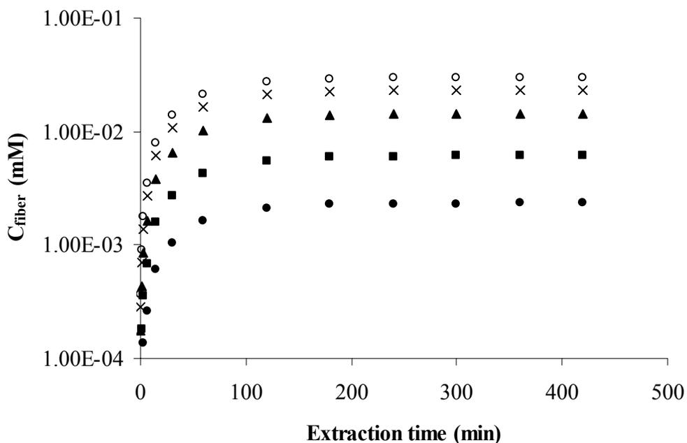
**Figure 5-4** Extraction profiles with different binding constants:  $8.9 \times 10^3$  (○),  $3.0 \times 10^4$  (×),  $8.9 \times 10^4$  (▲),  $3.0 \times 10^5$  (■) and  $8.9 \times 10^5$  (●).
