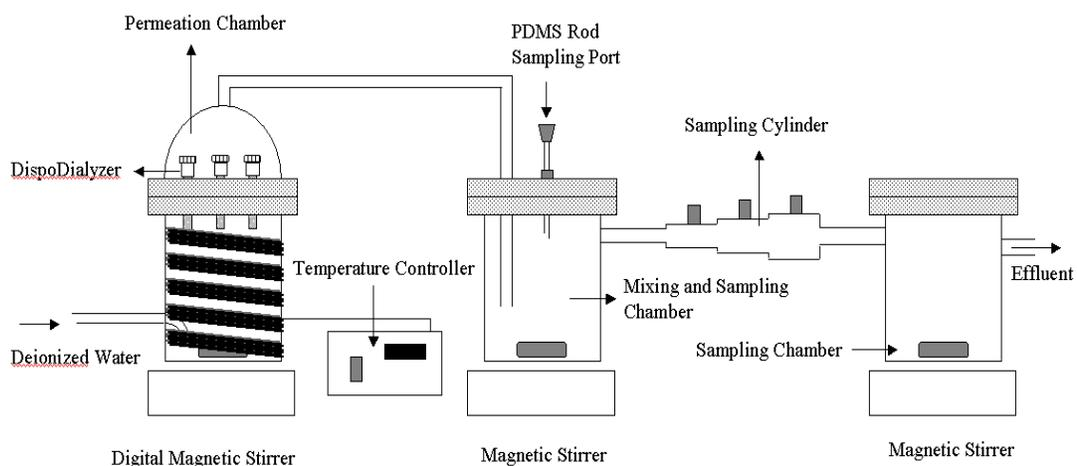
**Figure 3-3** Schematic diagram of the flow – through system.
