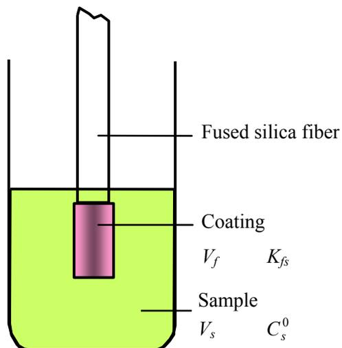
**Figure 1-1** Sample preparation with SPME.  $V_f$ , volume of fiber coating;  $K_{fs}$ , fiber/sample distribution coefficient;  $V_s$ , sample volume;  $C_s^0$ , initial concentration of analyte in the sample matrix.
