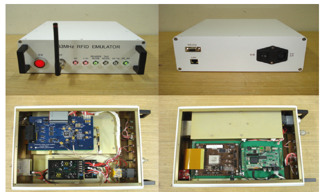
Fig. 9. View of the manufactured emulator for active RFID.
