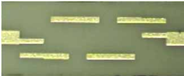
Fig. 2. Photograph of microstrip BPF
