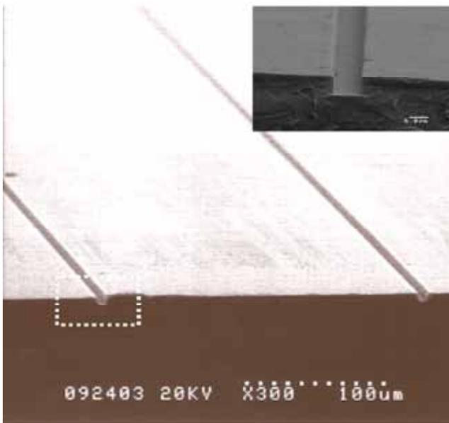
Fig. 4. SEM pictures of hot-embossed waveguide channels on a spin-coated PMMA thin film.
