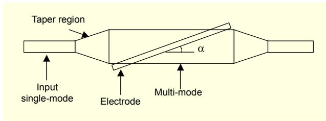
Fig. 1. A schematic layout of the fabricated VOA proposed by Noh et al. [2].
