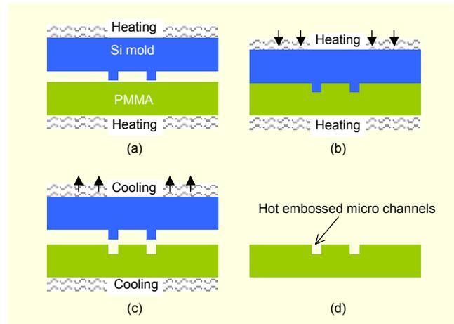
Fig. 3. An illustration of the hot embossing process: (a) a polymer and mold were heated above its glass transition temperature, (b) a mold was pressed into a polymer, (c) after adequate holding time the polymer was cooled down below its glass transition temperature and then the mold was lifted up, (d) well-defined micro channels were obtained.
