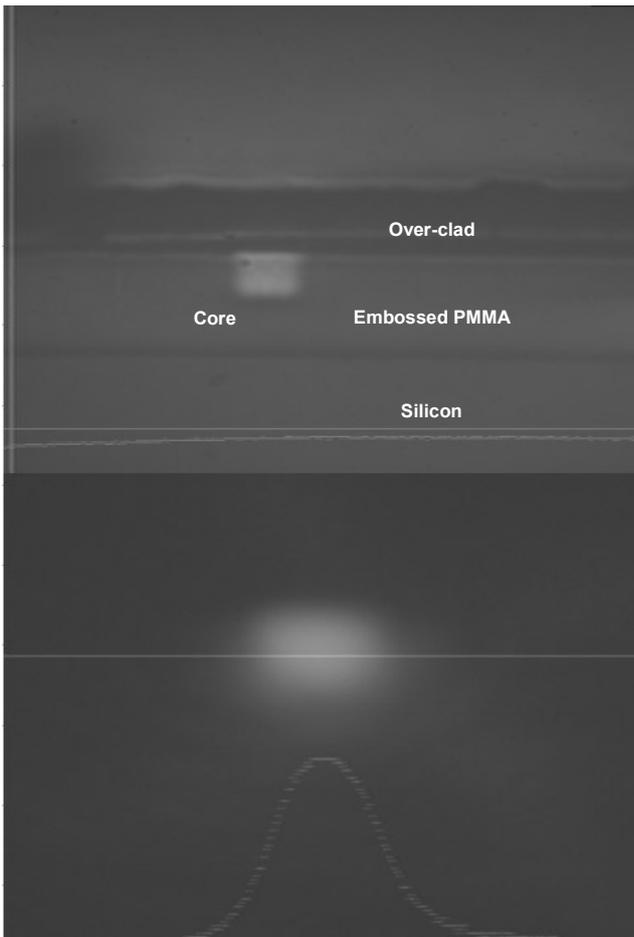
Fig. 5. A cross-sectional view of a fabricated polymer waveguide and a near-field pattern at a wavelength of 1.55  $\mu\text{m}$ .
