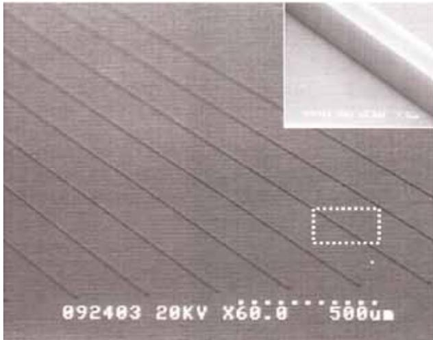
Fig. 2. A silicon mold for embossing polymer waveguide channels.
