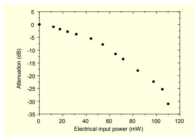
Fig. 6. Measured optical power attenuation according to applied electrical input power.
