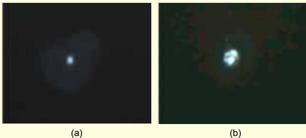
Fig. 6. Transmitted image of the 1.31  $\mu\text{m}$  light source at the end of the fabricated selenide fiber using (a) single mode and (b) multi-mode. The image was taken from a CRT monitor connected with an IR CCD camera.
