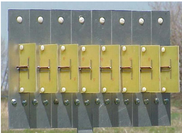
Fig. 8. Photograph of the printed dipole antenna array.
