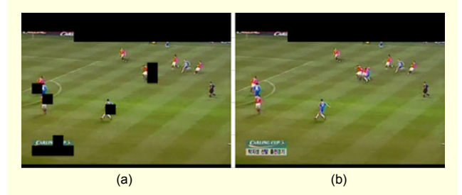
Fig. 7. (a) Ground block map (GBM) before filling holes. The black blocks are non-ground blocks. (b) GBM with holes filled.
