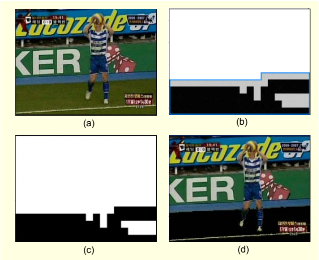
Fig. 12. (a) Original image, (b) original GBM , (c) EGB map (extended areas are denoted in gray), and (d) binary image with non-ground pixels in gray. Note that ground pixel detection is not conducted in white regions.
