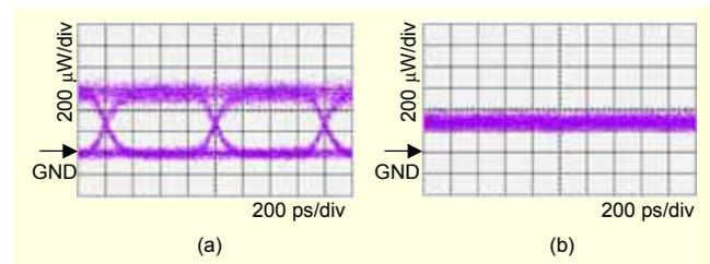
Fig. 4. Eye diagram of DCE #1 output when DCE #1 was coded with (a) Code#1 and (b) Code#2. Receiver bandwidth was 7.5 GHz for the eye measurement.
