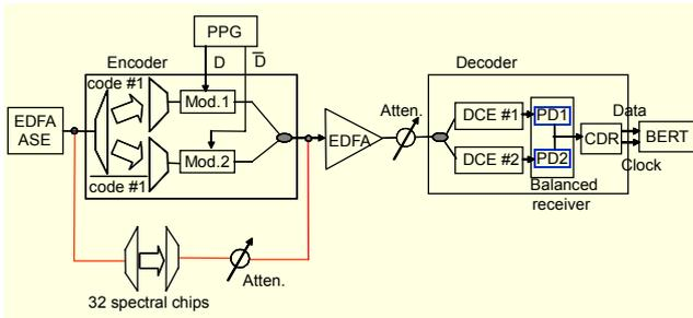
Fig. 2. Experimental set-up for bipolar spectral encoding CDMA.
