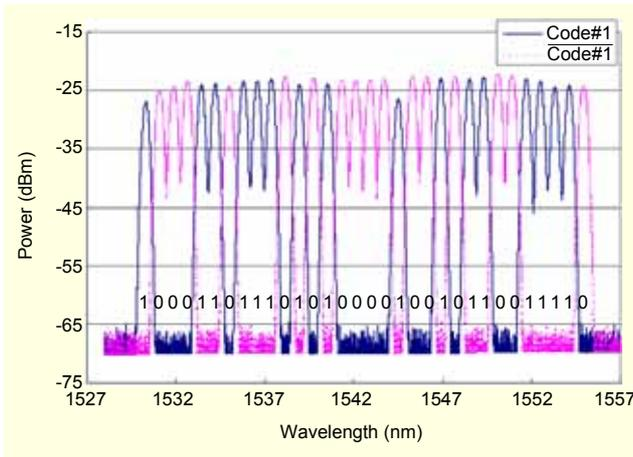
Fig. 3. Optical spectrum of encoder output coded with Code#1 and  $\overline{\text{Code\#1}}$ . Resolution bandwidth was 0.1 nm. The code sequence of Code#1 is depicted.
