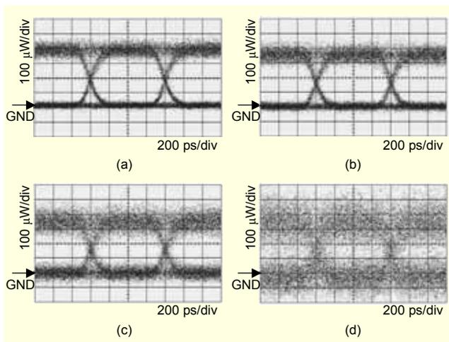
Fig. 5. Eye diagrams of DCE #1 outputs under the conditions of (a) one channel, (b) two channels, (c) four channels, and (d) eight channels. Receiver bandwidth was 7.5 GHz for the eye measurement.
