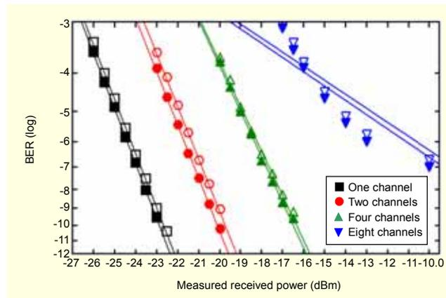
Fig. 6. BER performance with measured received power of balanced receiver when the number of channels was changed. BER data depicted with hollow symbols were the results after 80 km SMF transmission.
