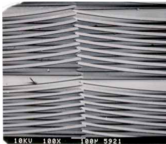
Fig. 4. Cross-sectional SEM image of micro-probe beam after the annealing process.
