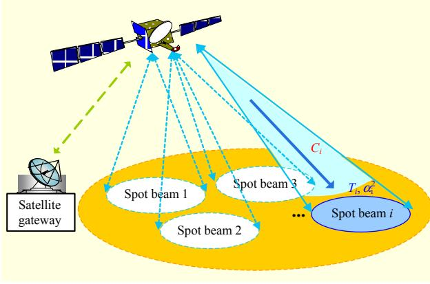
Fig. 1. System configuration of multi-spot-beam satellite.
