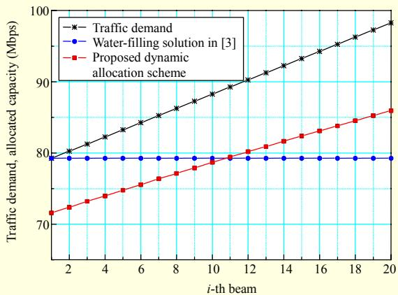
Fig. 3. Distribution of capacities for two resource allocations along spot beams having linearly increased distribution of traffic demand.
