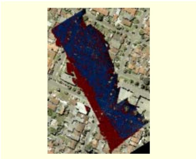
Fig. 9. Matched (blue) and unmatched-points (red) of the first surface displayed on an ortho-photo of the target area.
