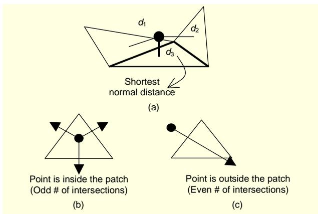
Fig. 5. Matching criterion 1: (a) shortest normal distance. Matching criterion 2: (b) projected point is inside and (c) outside the patch.
