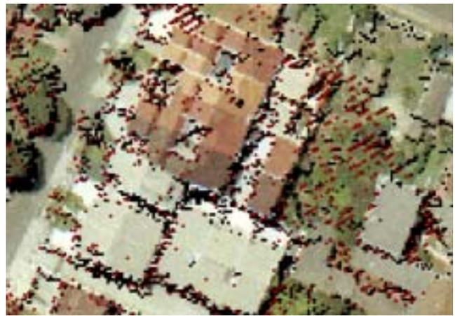
Fig. 10. Unmatched points (red) are mainly located along building boundaries and around areas with vegetation.
