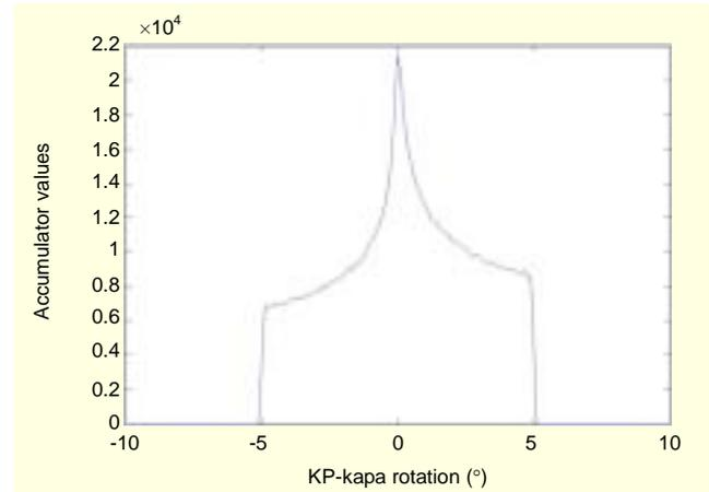
Fig. 3. An accumulator array with the peak indicating the most probable solution for the parameter in question.
