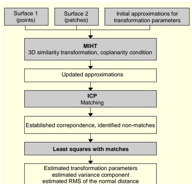
Fig. 6. Automated surface matching and registration algorithm.
