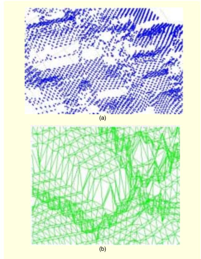
Fig. 8. Sections of (a) the first LIDAR surface represented by 44,156 points and (b) the second surface modeled by 45,520 triangular patches.
