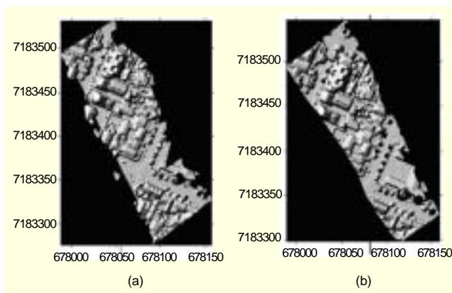
Fig. 7. Overlapping LIDAR range images over an urban area: (a) S<sub>1</sub> and (b) S<sub>2</sub>.
