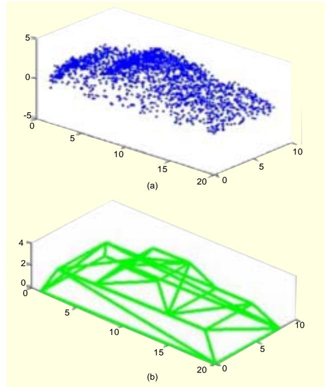
Fig. 1. Registration primitives for the proposed surface matching algorithm: (a) points for  $S_1$  and (b) triangular patches for  $S_2$ .
