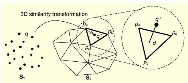
Fig. 2. Coplanarity condition describes the correspondence between a point in  $S_1$  and a patch in  $S_2$  after performing a 3D similarity transformation.
