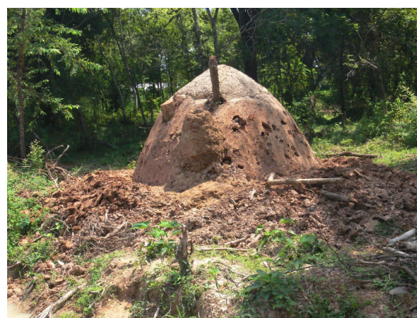
Figure 3 Termite mound for charcoal kiln. Base diameter and height of kiln were 2.4 m and 1.8 m, respectively. Termite species was unknown.
