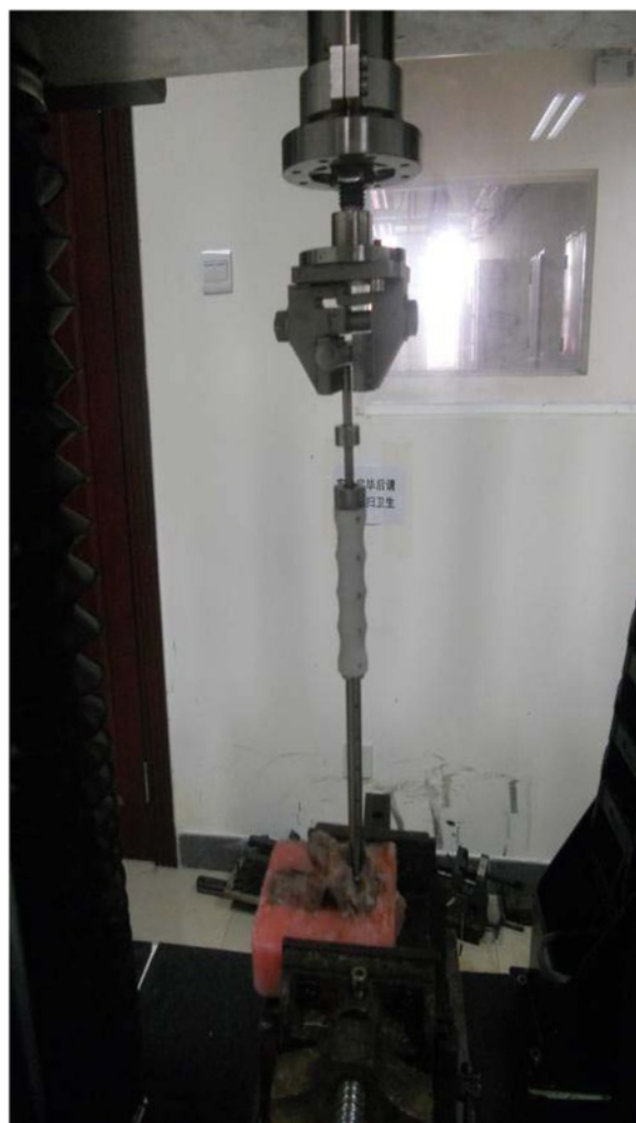
Figure 5 Device used for maximum insertion torque test.
