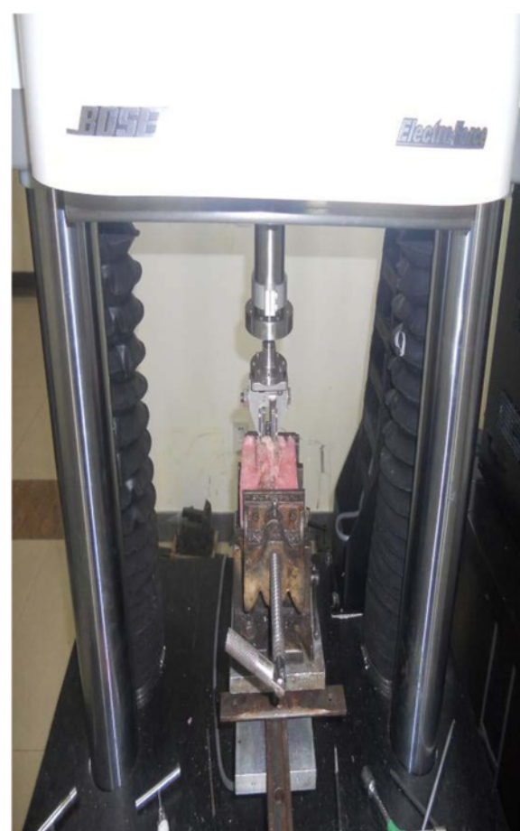
Figure 6 Device used for maximum pullout strength test.
