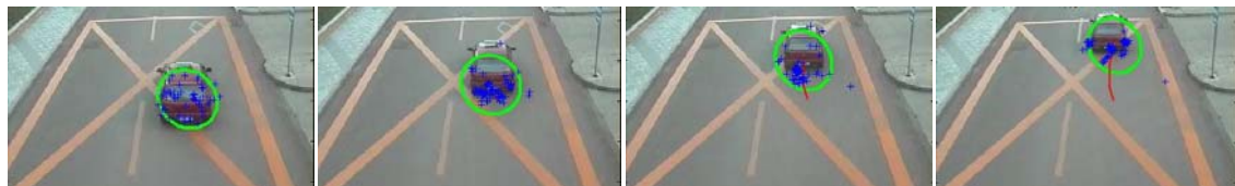
(b) Particle filtering tracking combined with SIFT by our method (Frames 10, 24, 39, and 56 are displayed)
