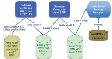
Aura OMI instrument observations of NO2 (Tropospheric NO<sub>2</sub>) in Level 2 (by orbit) format are acquired from the GES DISC and used to make multi-day Level 3 global grid for visual display.
