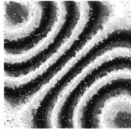
Fig. 2. Cubic image with 5% speckle noise. SNR: 9.91dB.
