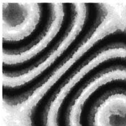
(c) Denoised image via BPDN with \ell^1 data fidelity term using an overcomplete DCT dictionary. SNR: 25.62
