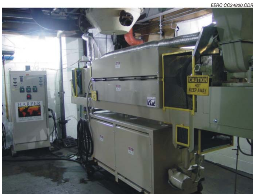
Figure 21. The rotary kiln reactor system installed in the EERC pilot plant.
