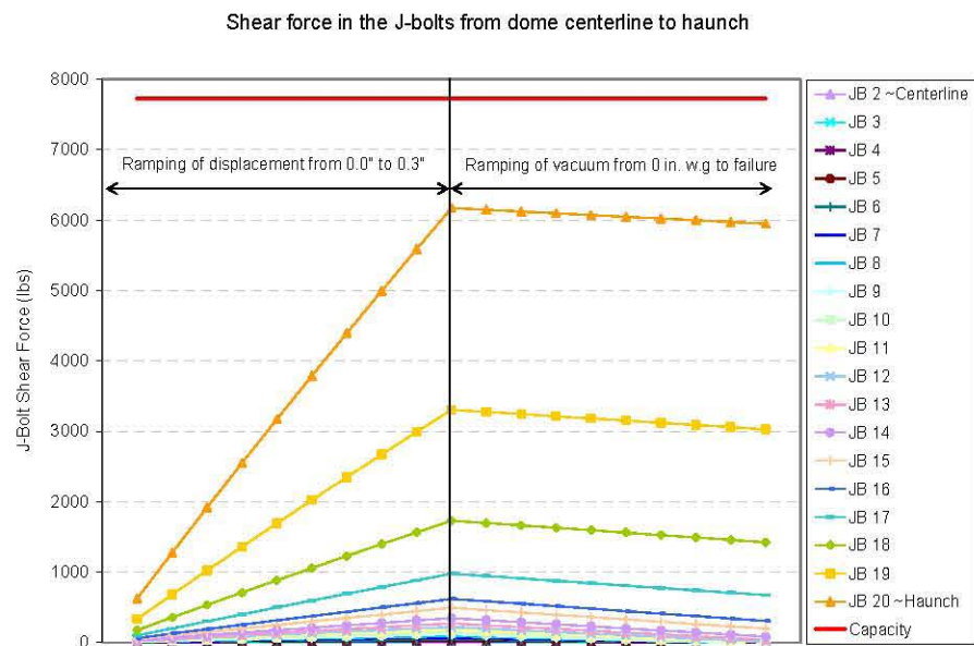
Figure 6-18. Shear Force Histories (for J-bolts from the dome centerline to the haunch) for the AP Tank with 0.3 Inch Axial Compression, 25-Inch Waste Height, and Increasing Vacuum Load
