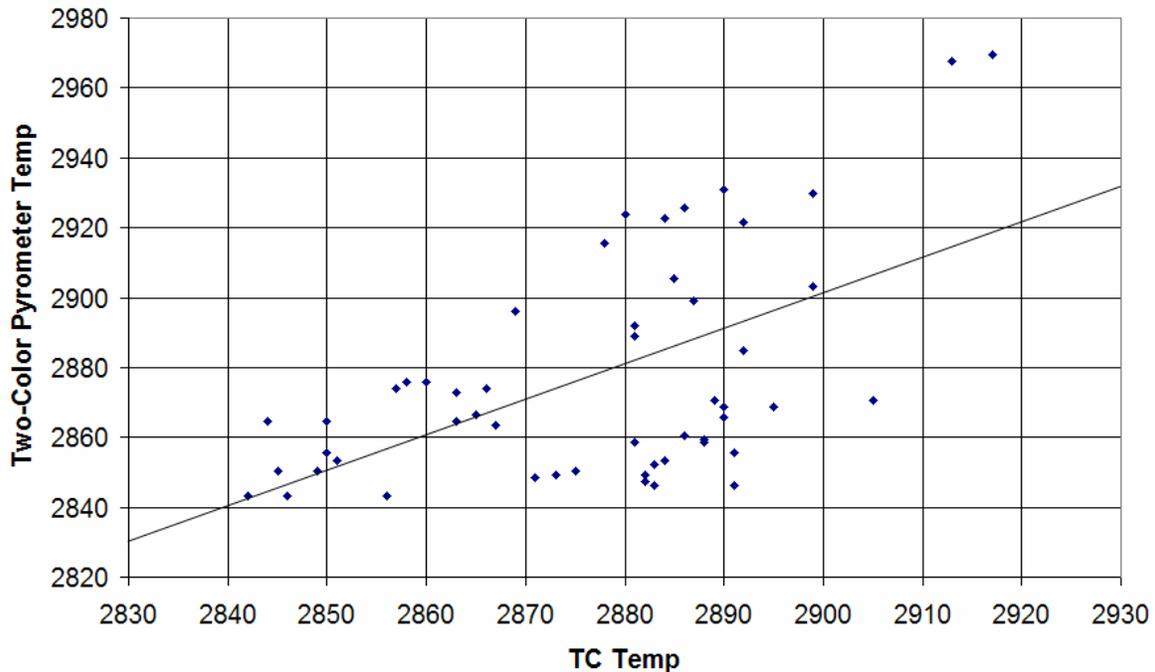
**Figure 5. Thermocouple temperature plotted against the temperature observed with the two-color pyrometer for the same heat.**
