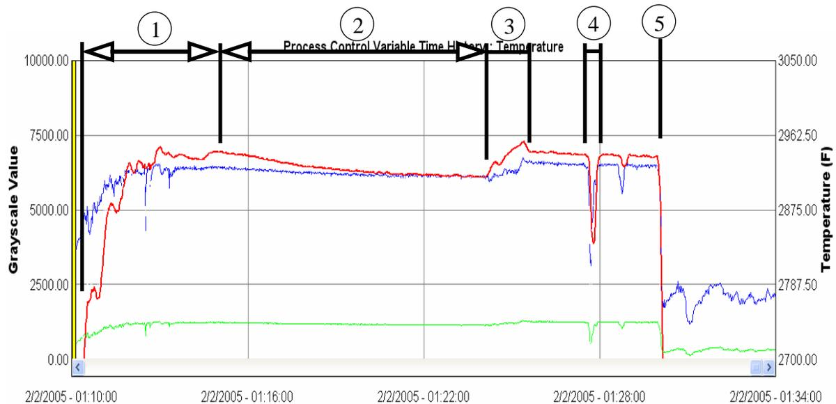
**Figure 3. Typical intensity and temperature traces for a complete heat in which no oxygen was added early in heat.**
