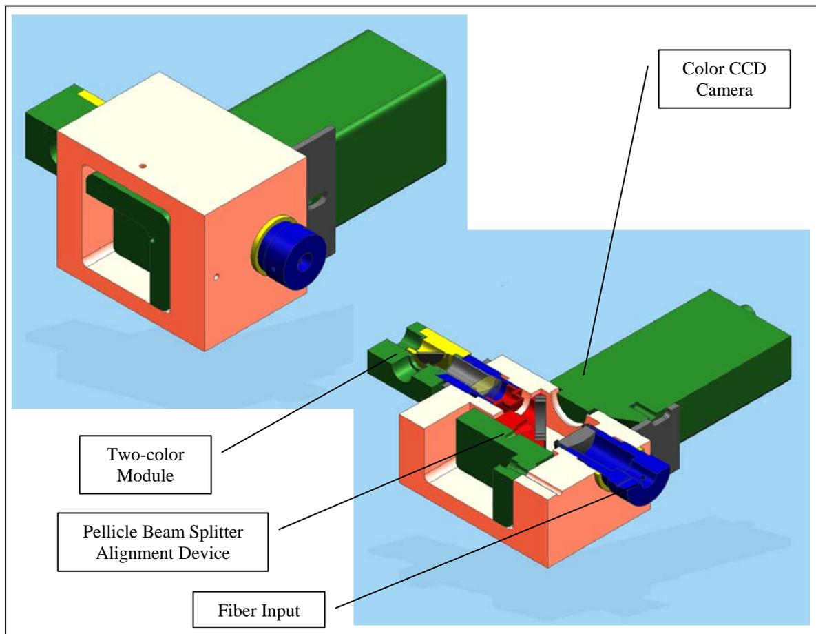
**Figure 1. Opto-mechanical design illustrated in 3-D CAD. System integrates fiber input, two-color pyrometer and color camera for imaging.**
