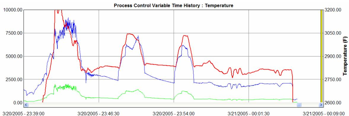
**Figure 4. Typical intensity and temperature traces for a complete heat in which multiple additions were made.**
