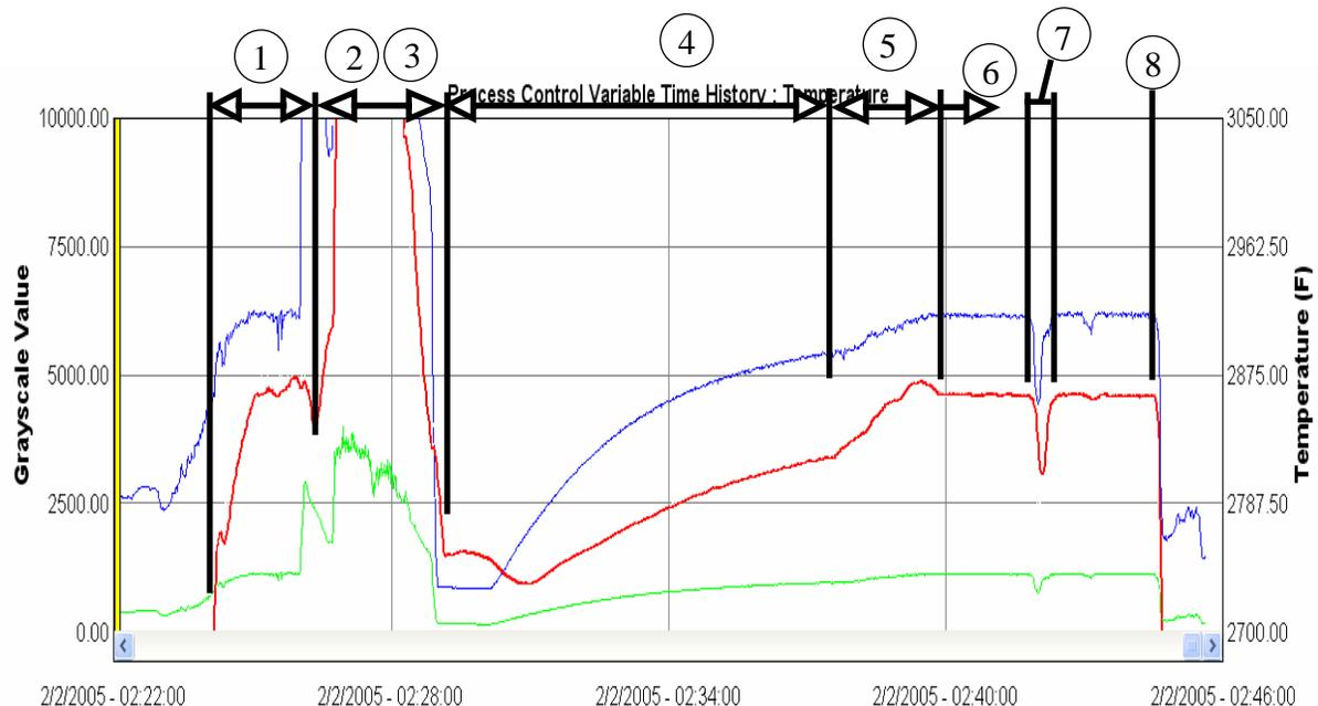
**Figure 2. Typical intensity and temperature traces for a complete heat in which oxygen was added near the beginning of the heat.**
