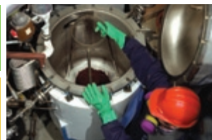
This pretreatment reactor hydrolyzes hemicellulose and solubilizes some lignin. The pressurized hot wash process separates these materials before they can reprecipitate. This system uses dilute sulfuric acid at increased temperature and pressure, but pressurized hot wash may work well with any pretreatment system.
