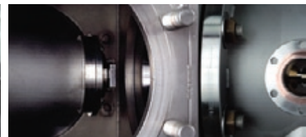
This pretreatment reactor hydrolyzes hemicellulose and solubilizes some lignin. The pressurized hot wash process separates these materials before they can reprecipitate. This system uses dilute sulfuric acid at increased temperature and pressure, but pressurized hot wash may work well with any pretreatment system.
