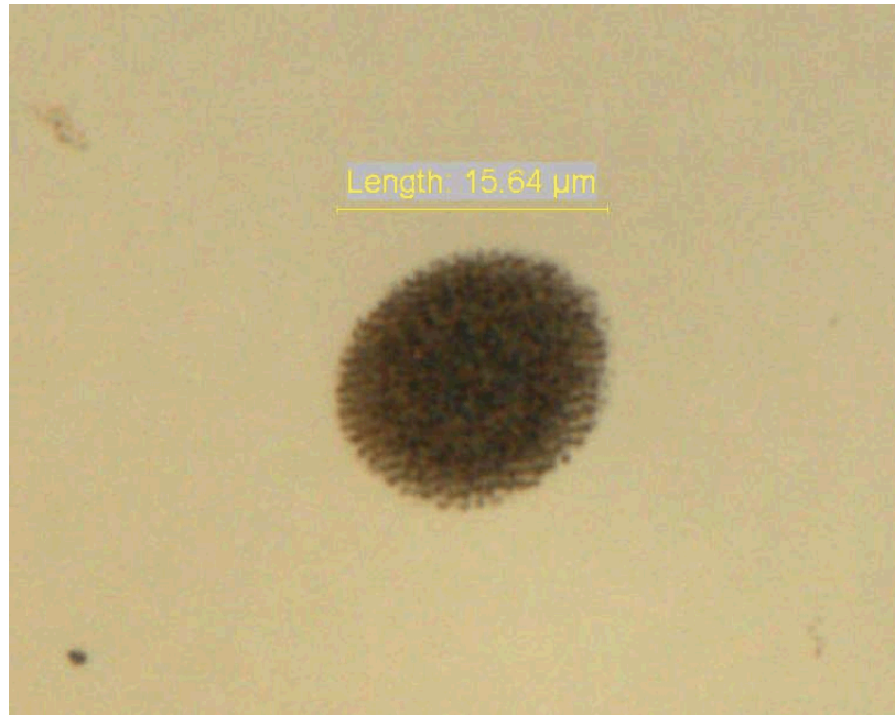
Figure A1. Optical micrograph of a laser damaged region of a GaAs wafer
