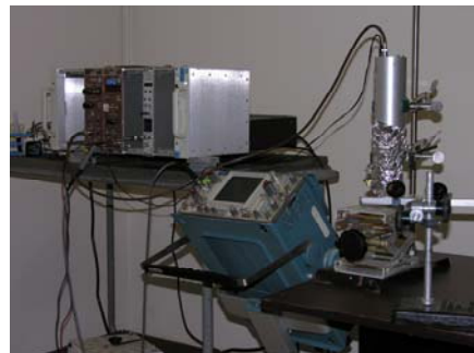
Figure 7 – Scintillations produced within the paint film by the alpha source were detected with the PMT, passed through a pre-amplifier on the base of the PMT tube, counted by a pulse counting network.
