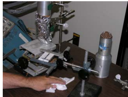
Figure 6 – The painted glass slides were held in close proximity to the face of a standard photomultiplier tube (PMT), with the glass slide facing the PMT, and the exposed paint film facing the Pu-239 alpha source.
