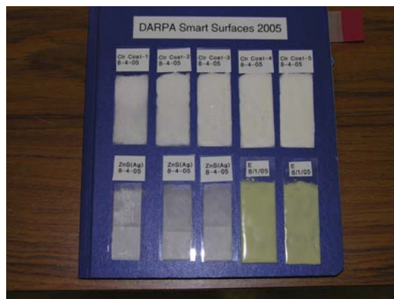
Figure 3 – Surfaces coated with scintillating paints. In this specific case, the pigment used in the paint is Ag-doped ZnS, which scintillates when bombarded by alpha particles.
