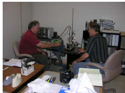
Figure 8 – This photograph shows nuclear chemist James Brunk using the oscilloscope to validate the PMT signal prior to pulse counting.
