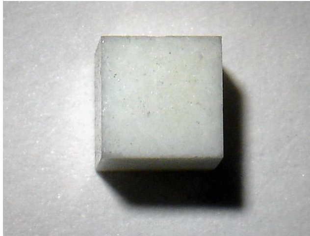
Figure 8: Photograph of a typical sample used for creep measurements (4x4x4 mm).
