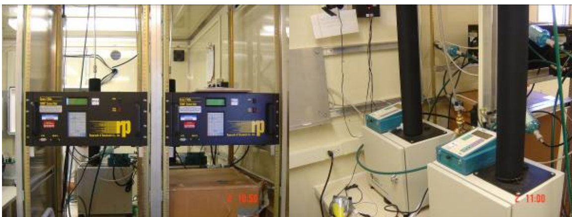
Figure 8. Left photograph: The front panels of PM 10 (right on the left photograph) and PM 2.5 (left on the left photograph) of TEOM. Right photograph: The measurement units of TEOM and DUSTTRAK on top of them.
