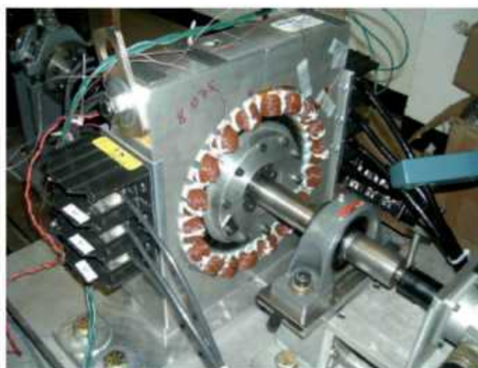
Fig. 16: View of prototype SPM2 machine during testing at UW-Madison
