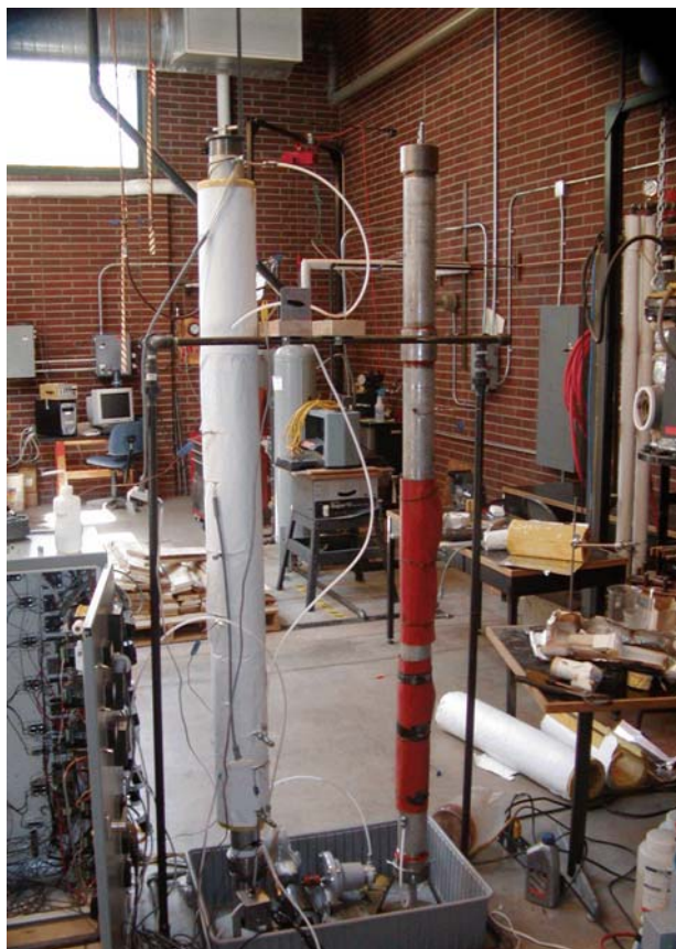
Figure 18. Columns with and without insulation. Heaters (two of four) are shown on right column.
