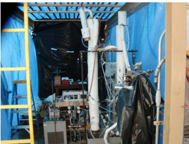
Figure 23. Equipment set up at particleboard facility. Sampling line from Figure 22 enters at right.
