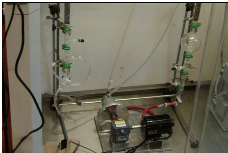
Figure 13. Lower part of columns without insulation with pump.
