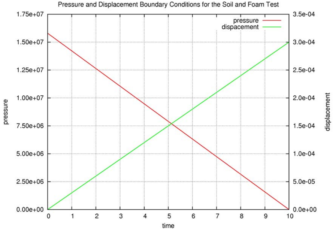
Figure 12: Boundary conditions for the soil and foam test problem.
