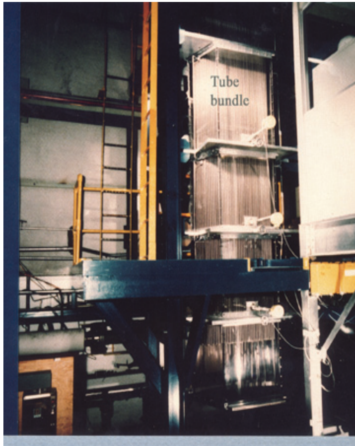
Figure 1. Example of a large separate-effects apparatus for the steam generator feedwater distribution and flooding experiments conducted at WRRTF.
