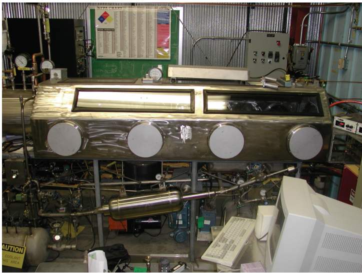
Figure 11. NaK flow loop located at the MFC Engineering Laboratory.
