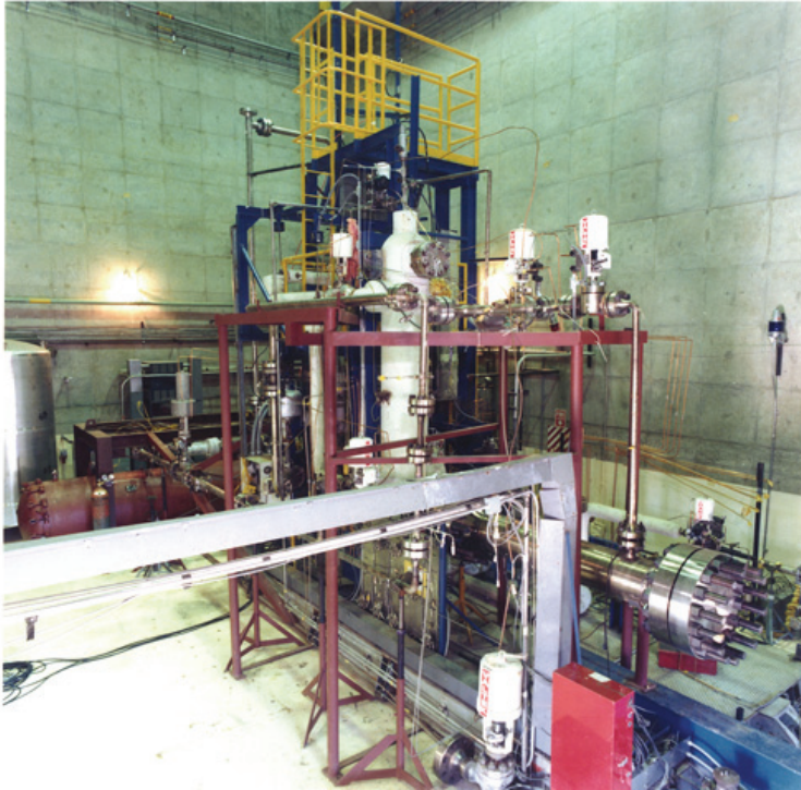
Figure 2. Steam-Air-Water (SAW) flow loop formerly located at WRRTF. Yellow ladder indicates size of apparatus.
