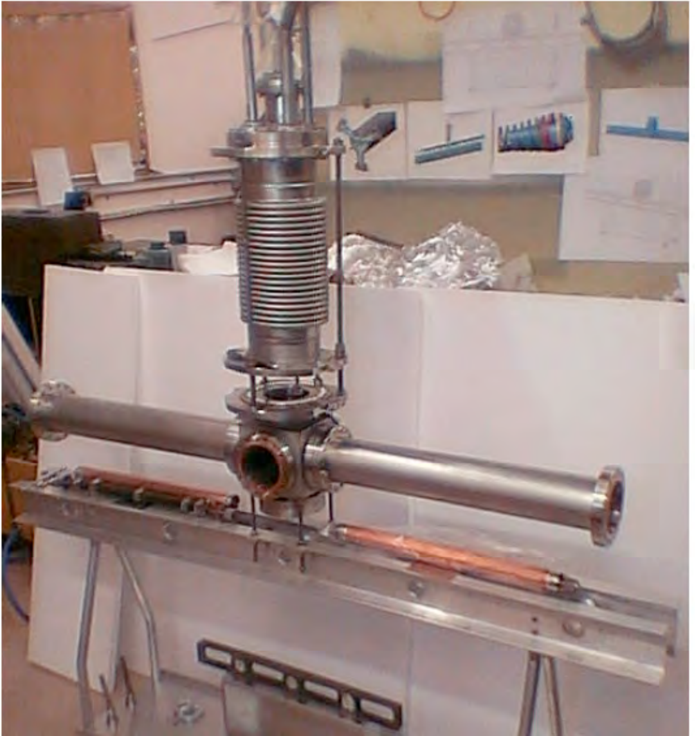
Fig. 8. 1m long model of an undulator cryostat for testing with 40 cm model cores waiting for assembly Extensive references will be found in the appended PAC 2007 paper WEZAB01.
