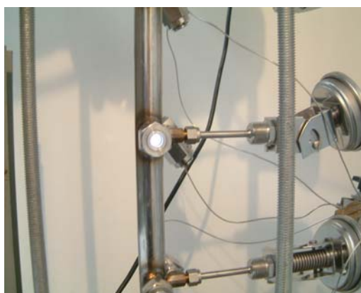
Figure 3.1. Corona discharge as seen through a view port
