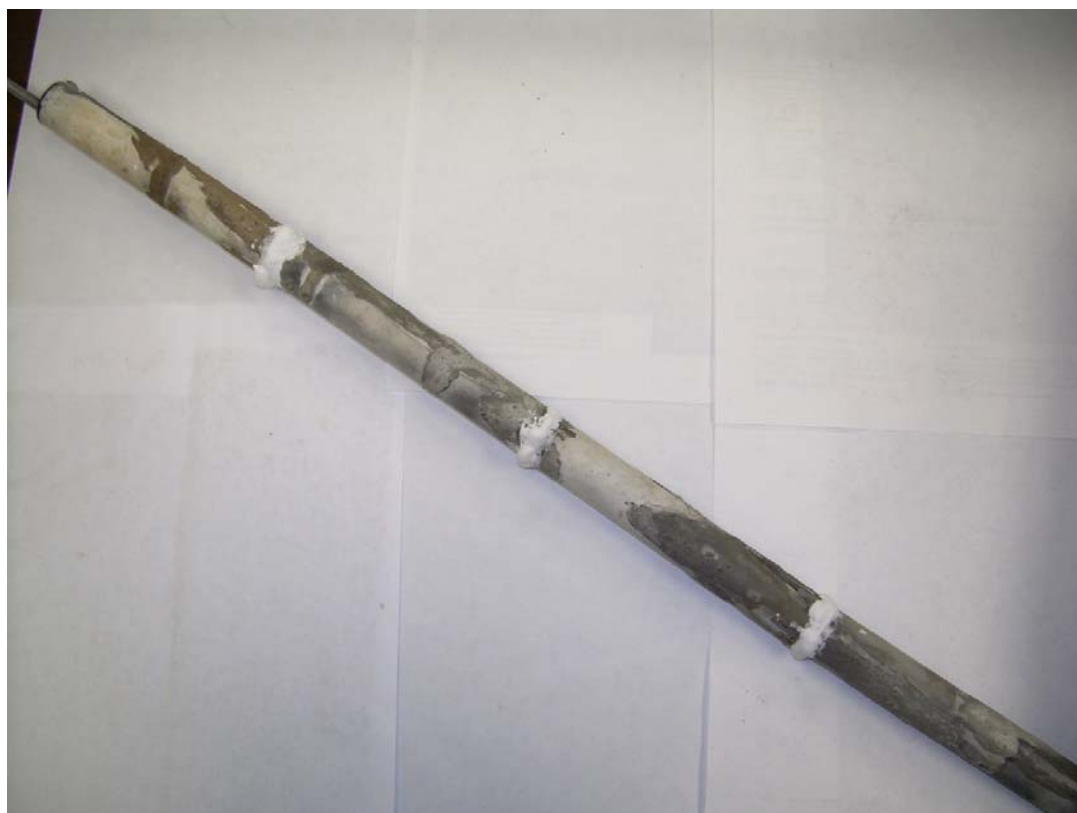
Figure 4.2. Vanadium-infiltrated alumina membrane tube
