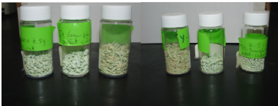
Figure 42. Selected nickel and molybdenum impregnated Al-SBA-15 catalysts extrudates
