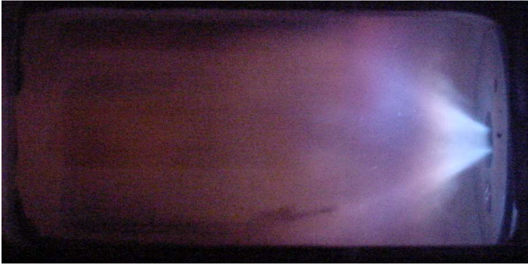
Figure 25: CO Flame Anchored in nozzle.
