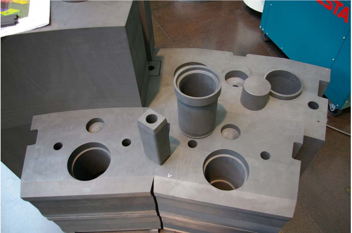
Fig. 3. PBMR DPP test parts assembly.
