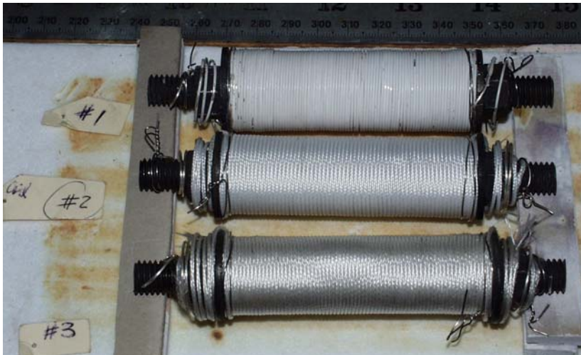
Fig. 1, 0.5" dia.x3"L. coils after winding.
