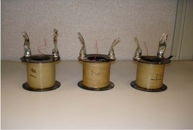
Fig. 7, Typical Coils after Heat-treatment and Epoxy VPI
