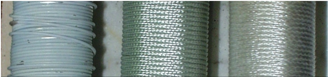
Fig. 2, Coil Insulation after heat-treatment
