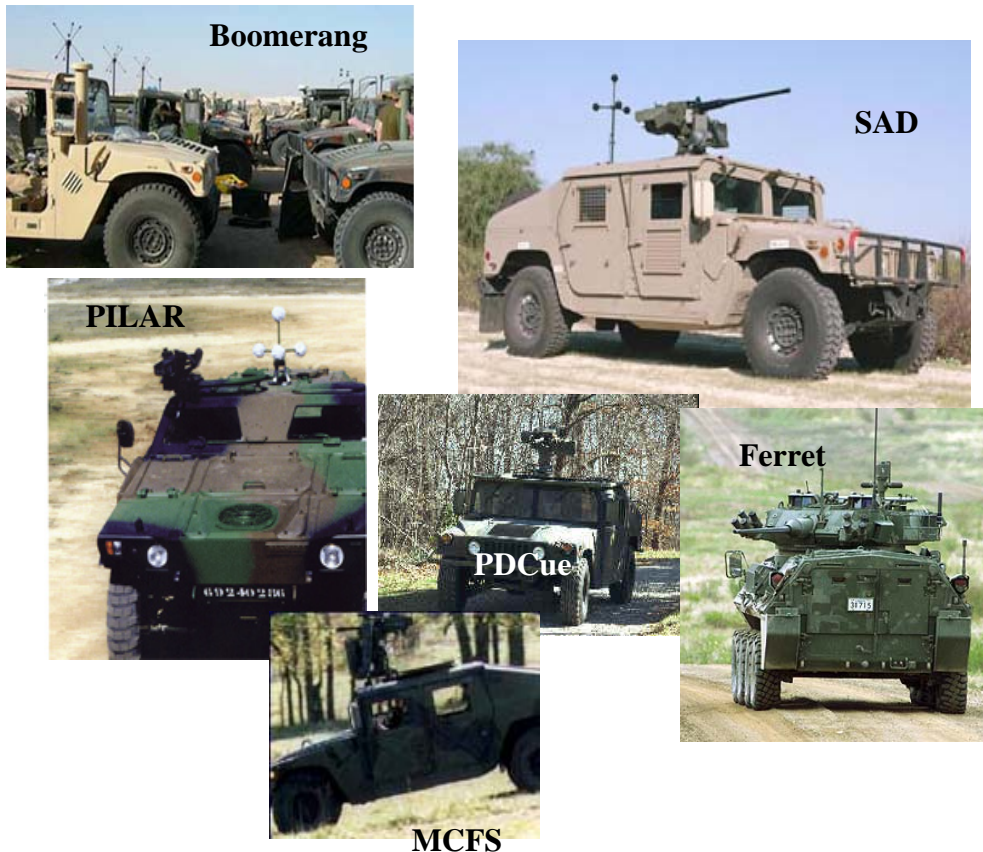
Figure 3. Examples of sniper detection systems employing standard microphones in 3D array format.
