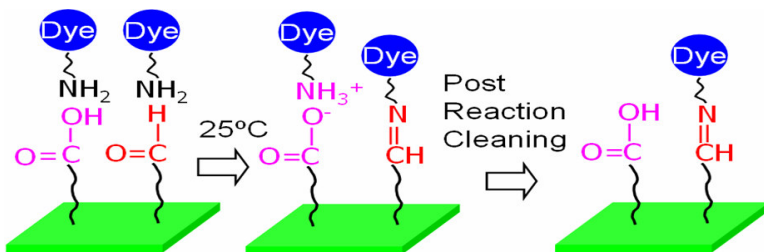
Fig. 6 The post reaction cleaning procedure is effective to remove ionically bonded dyes on the surface. The presence of carboxyl groups on the surface will not affect the detection of aldehyde groups using amino modified dye.[7]
