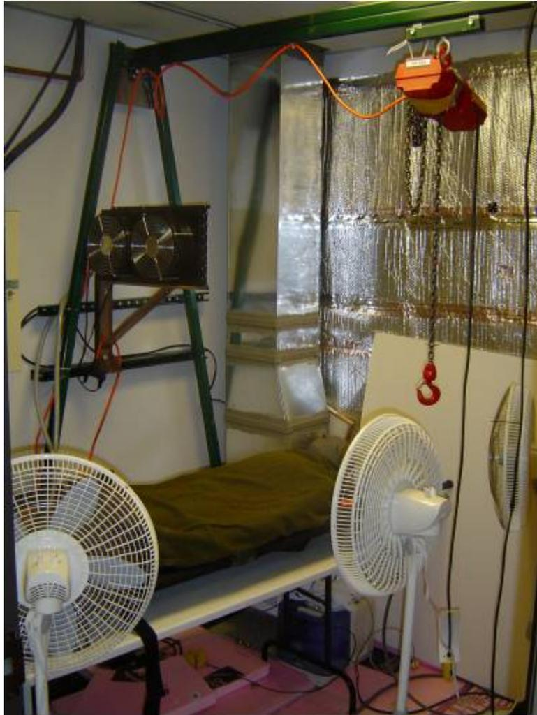
**Figure 40. NREL's Manikin Environmental Chamber**
