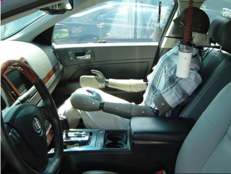
Figure 19. ADAM testing a W.E.T. ventilated seat
