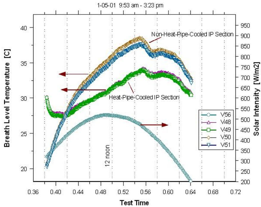
Figure 22. Temperatures of a heat-pipe-cooled and non-cooled IP
