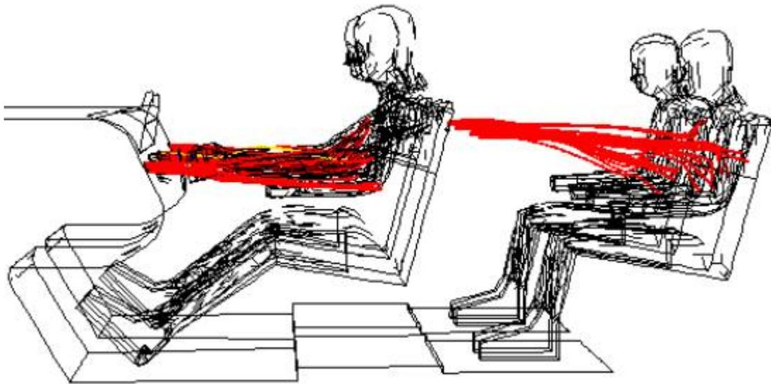
**Figure 6. Flow path lines from body coolers**
