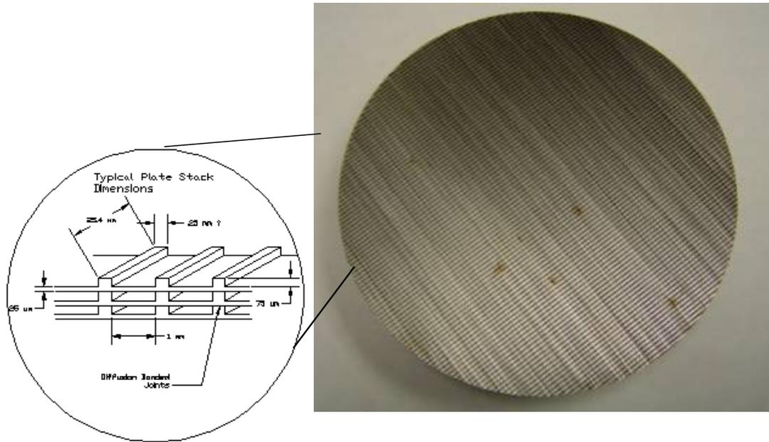
**Figure 25. Microchannel regenerator prototype for a thermoacoustic generator**
