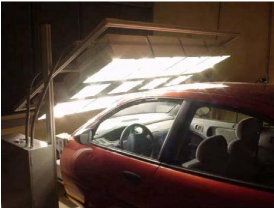
**Figure 18. Vehicle Climate Control Laboratory with solar lamps**
