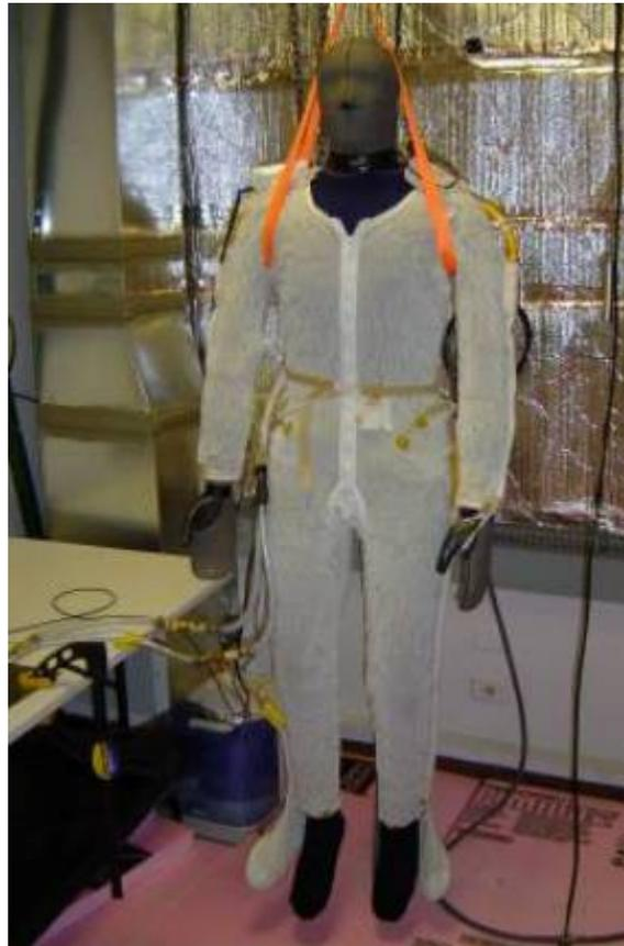
**Figure 36. ADAM in a NASA Liquid Cooling Garment**
