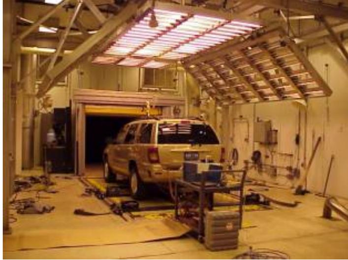
**Figure 44. Chrysler Environmental Test Cell with IR lamps**
