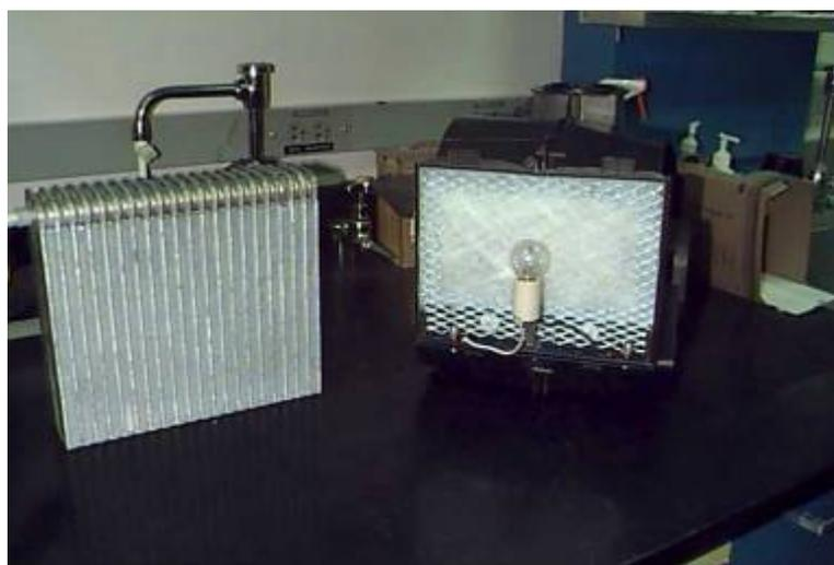
**Figure 29. A prototype photocatalytic air-cleaning system**
