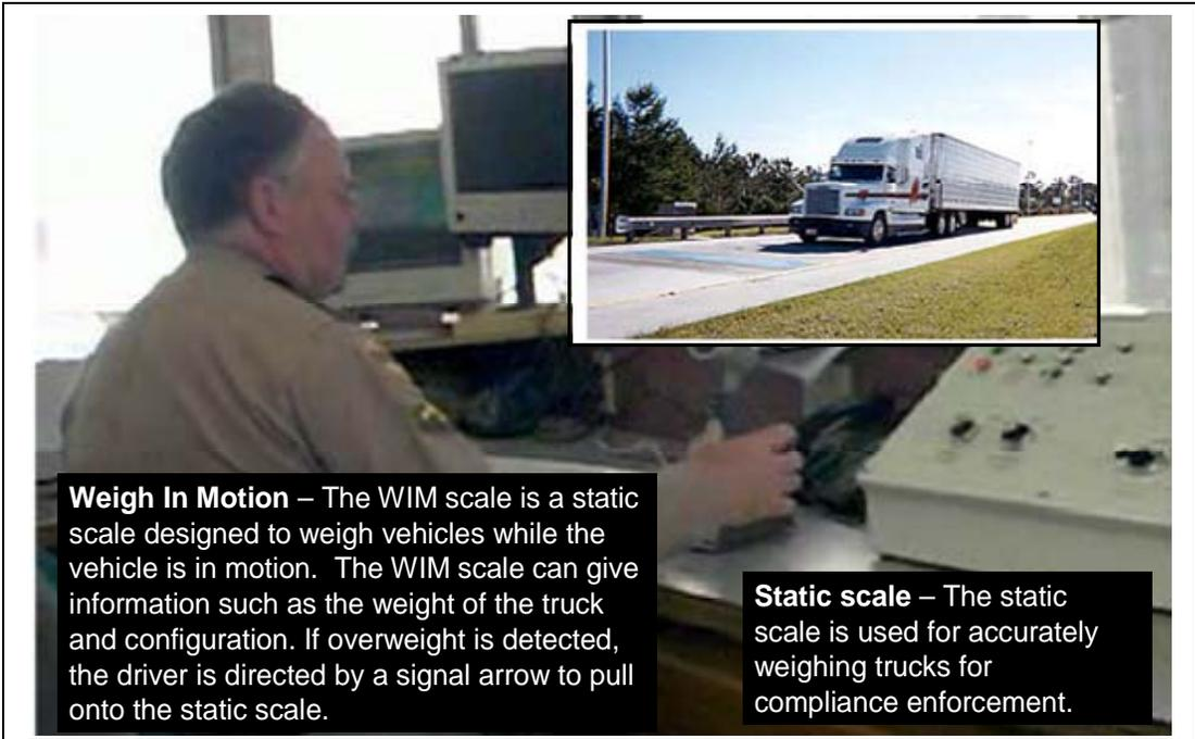
**Figure 11. Weigh-in-Motion and static scales for vehicle weight.**
