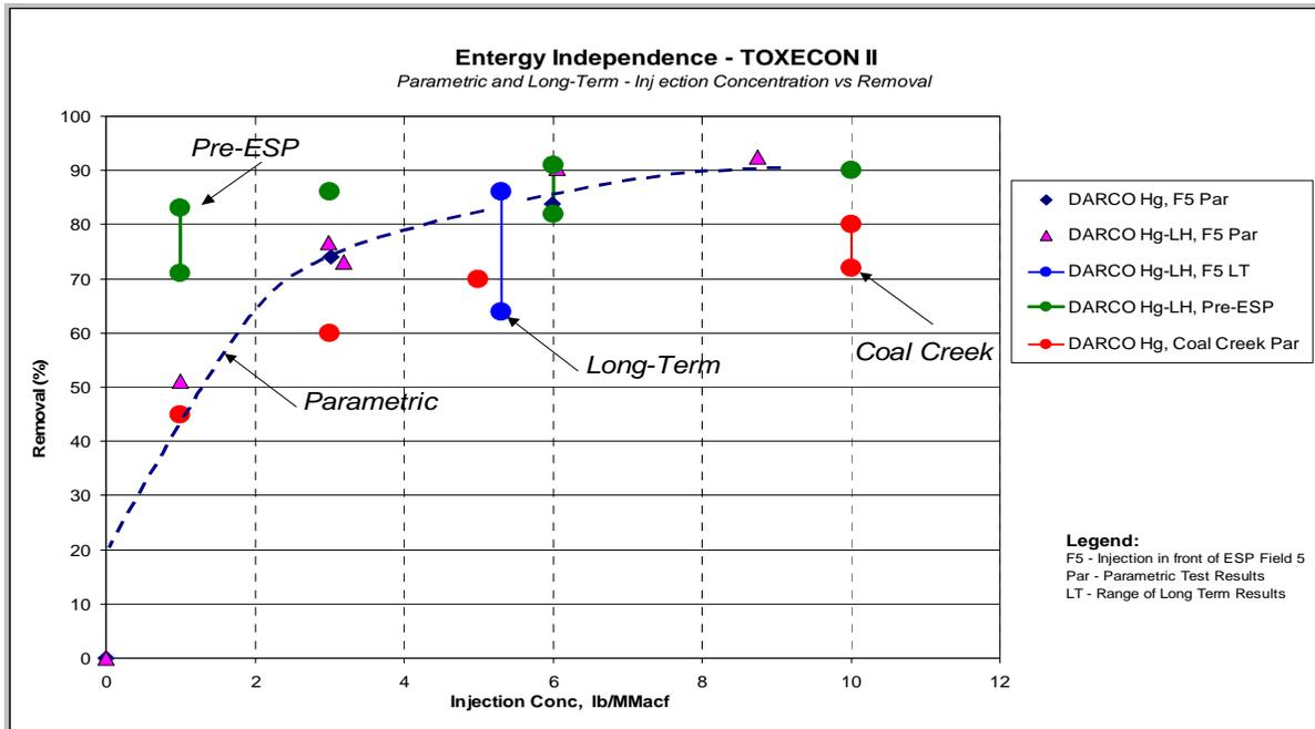
**Figure 7. Varying Mercury Removal Performances.**
