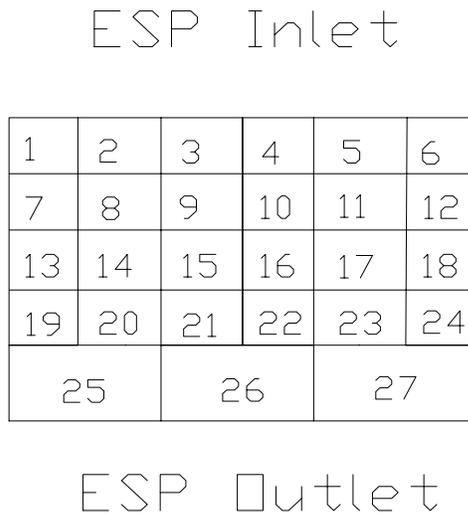
**Figure A-2. Single ESP Box Electrical Field Configuration.**
