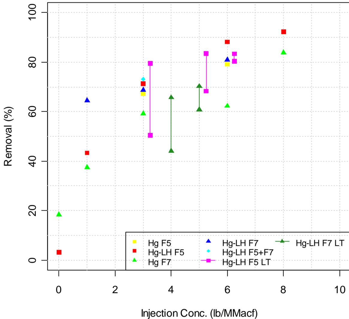
**Figure 6. Comparison of DARCO® Hg and Hg-LH Performance from Parametric and Long-Term (LT) Tests at the Mid-ESP (F5) and Rear-ESP (F7) Injection Locations.**
