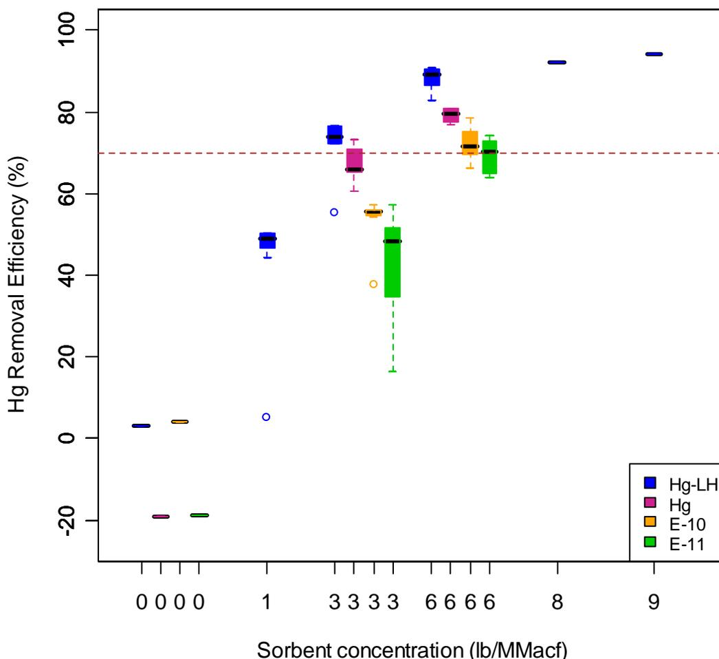
**Figure 5. Comparison of Sorbent Performance During the First Set of Parametric Tests (mid-box injection, field B-7 down, field B-3 low/no power, dashed line at 70%).**
