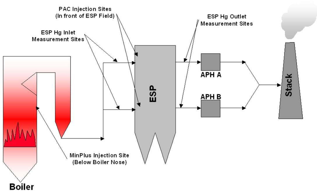
**Figure A-3. Council Bluffs Unit 2 Plant Configuration and Potential Injection Sites.**
