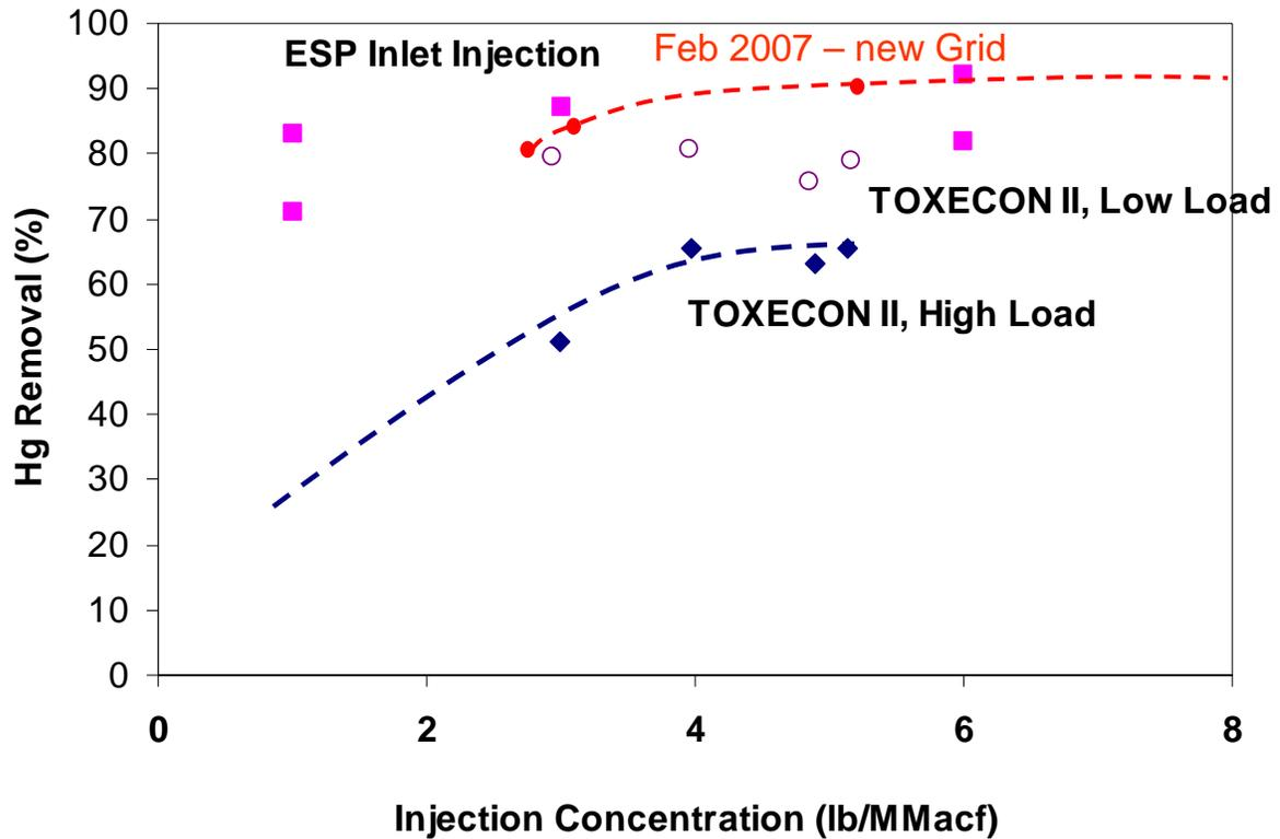
**Figure 10. Mercury Removal Comparison of Injection Location and Grid Design.**
