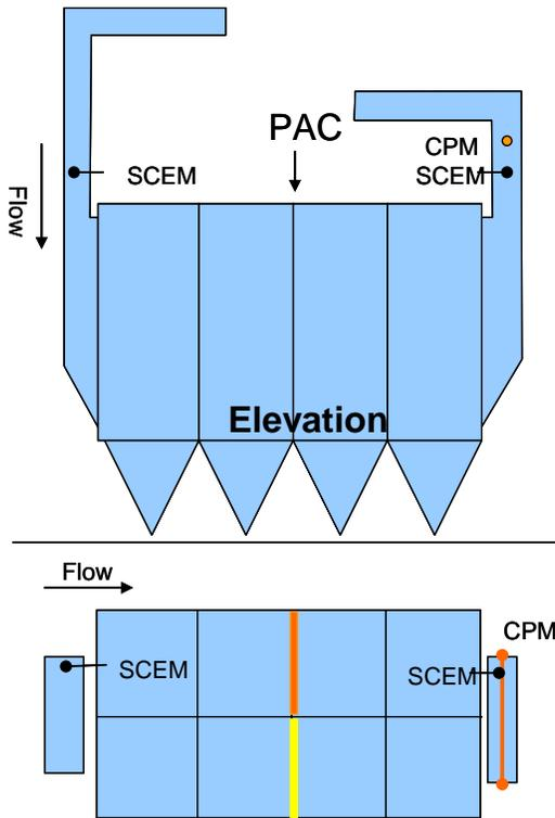
**Figure 3. West Half of the Unit 2 B ESP (1/8 of the Unit 2 Flue Gas) with Mid-ESP Injection and Inlet/Outlet Monitor Locations Indicated.**
