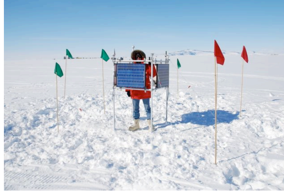
The omnidirectional solar array of the prototype station on the Ross Ice Shelf, Antarctica
