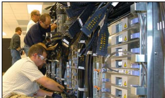
Engineers installing the Blue Gene/P supercomputer
