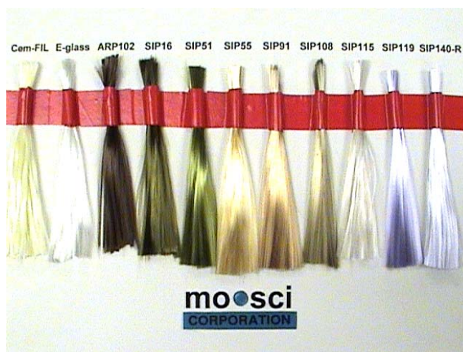
Figure 2. Samples of continuous Ca-Fe-phosphate fibers manufactured at MO-SCI Corp. The color is dependent upon the glass composition. The commercial silicate glasses CemFIL ® and E-glass, are shown on the left.
