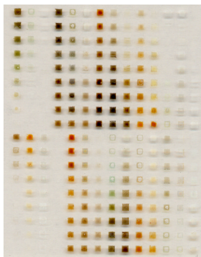
Figure 6: FTO slide printed with binary combinations of eight metals
