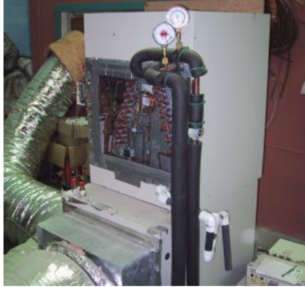
Figure 14: I-HVCD Prototype Coil Assembly
