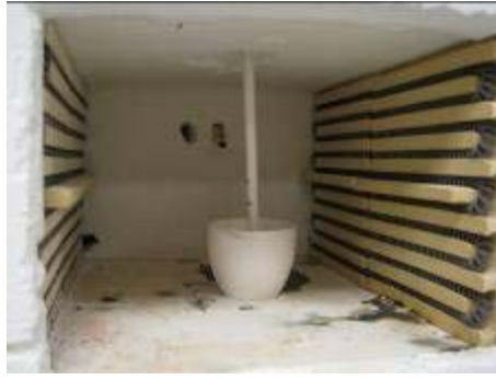
Figure 30: Experimental setup for corrosion experiment. The alumina tube containing the fiber sensor is immersed in sodium carbonate in the crucible
