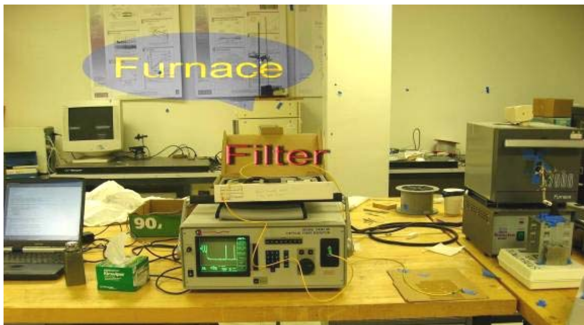
Figure 24: System setup for 1000°C testing
