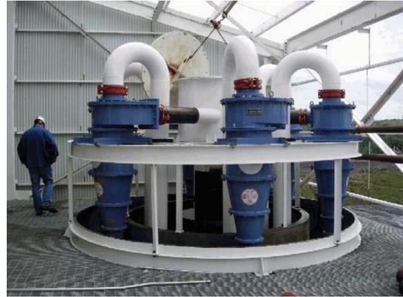
Figure 40. Classifying cyclones used to provide a 100 mesh cutsize.
