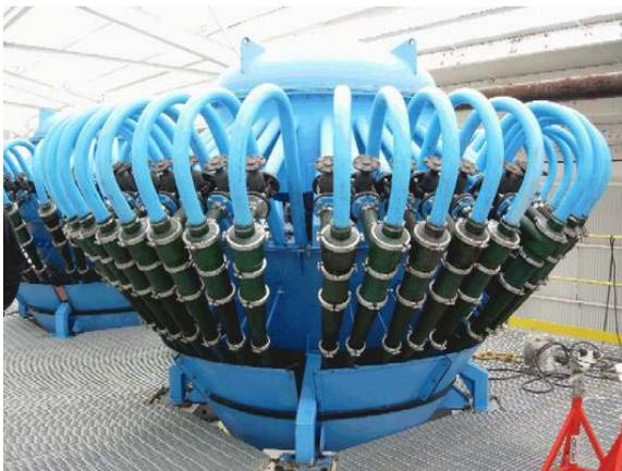
Figure 37. Deslime cyclones used to perform a nominal 325 mesh cutsize.
