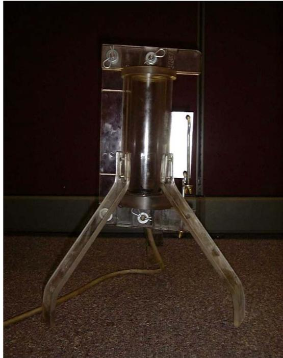
Figure 6. Photograph of the 3.5-inch diameter pressure filter.
