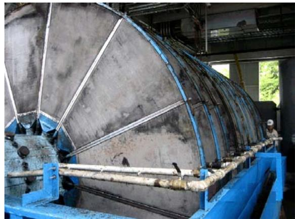
Figure 42. Bank of disc filters used to dewater the fine coal froth product.
