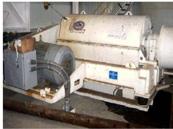
Figure 38. Screen-bowl centrifuge used to dewater 100x235 mesh product.
